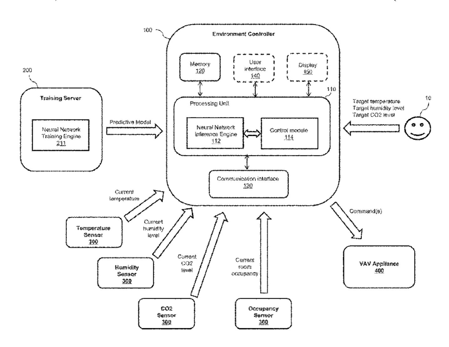
characteristic value and the at least one set point. The environment controller transmits the one or more commands to the controlled appliance.
