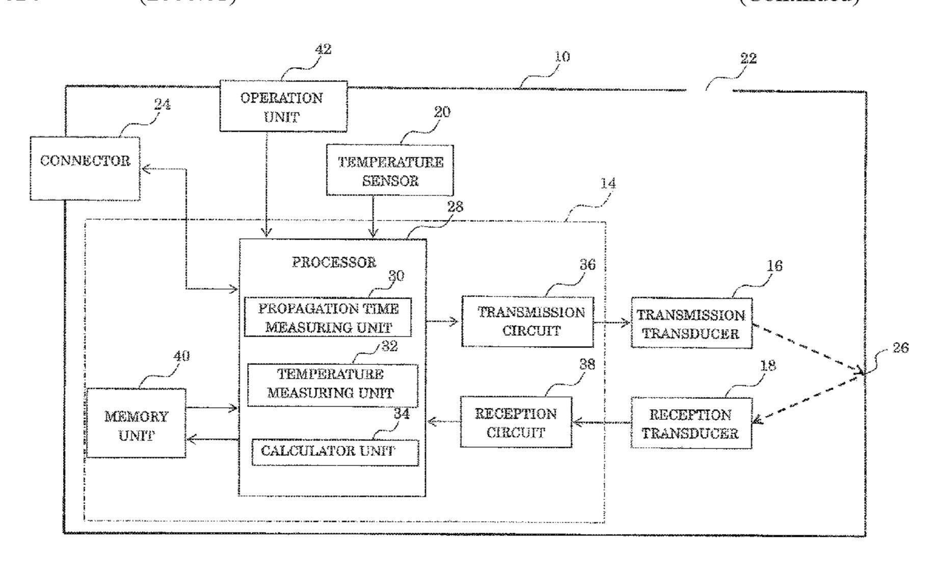
calculating process is executed for each of a plurality of temperature conditions under which the temperature of a reference gas inside the housing differs. A temperature compensation table in which the temperature of a gas to be measured is associated with a temperature compensation value relating to the temperature is obtained on the basis of the temperature replacement fluctuation values obtained under each temperature condition.
