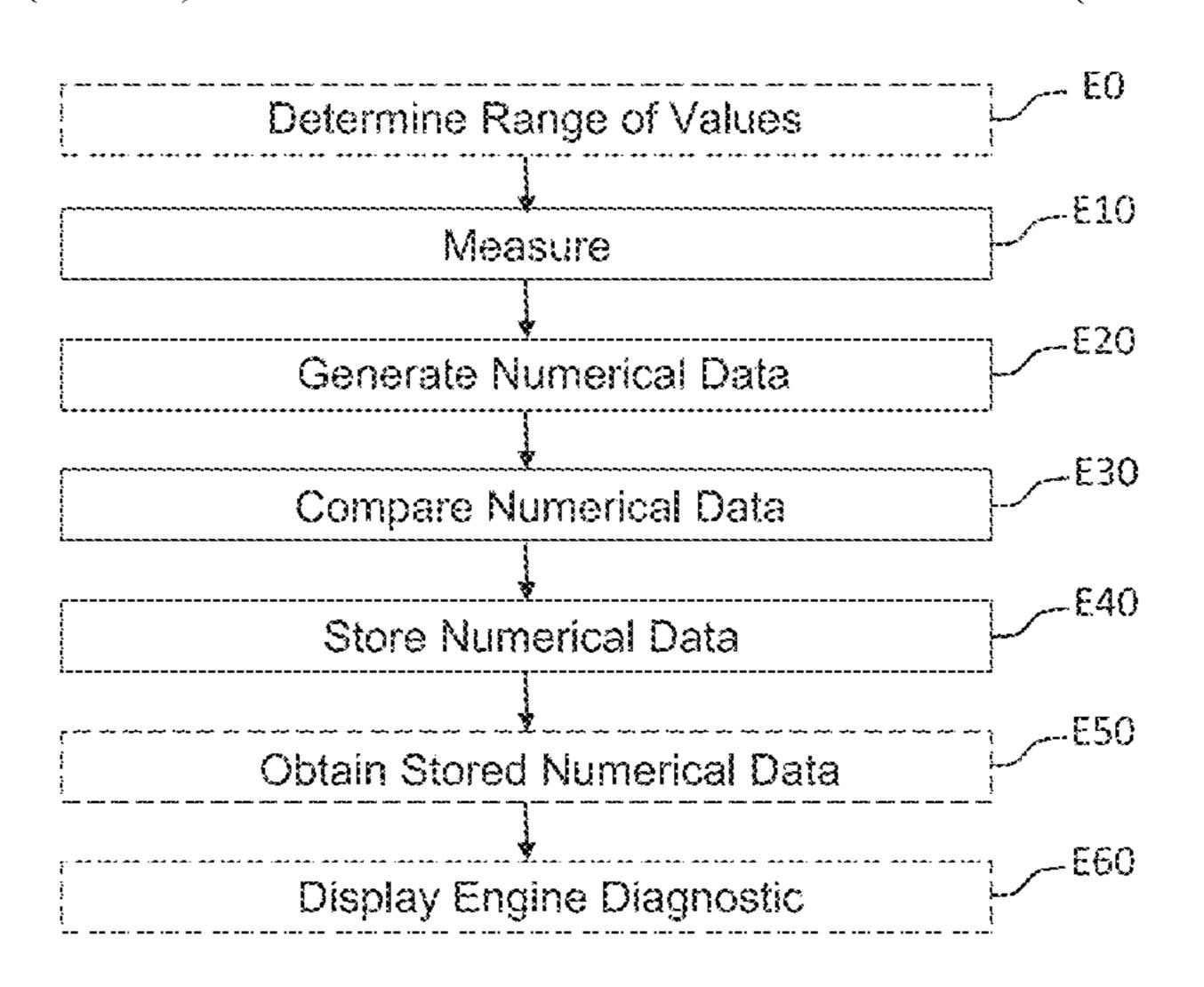
measuring sensor (110) to transmit at least one digital datum representative of the measured value of the parameter to the analysis computation means (140) and a step for using the analysis computation means (140) to compare said digital datum with a predetermined range of values representative of an operation of the anti-pollution system according to a predetermined standard.
