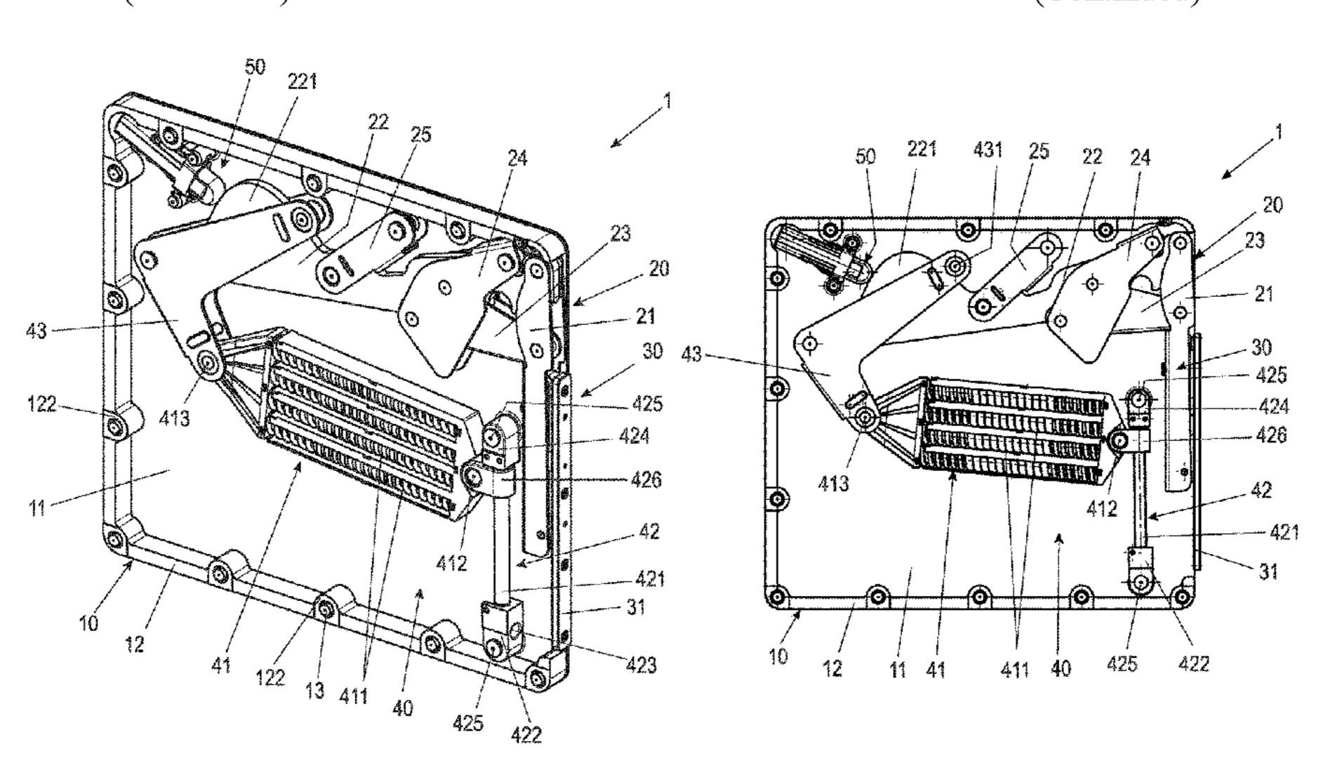
adjustable via an adjusting element having a tool receptacle. The tool receptacle is accessible through a front-side opening in the furniture board and/or the flap fitting.
