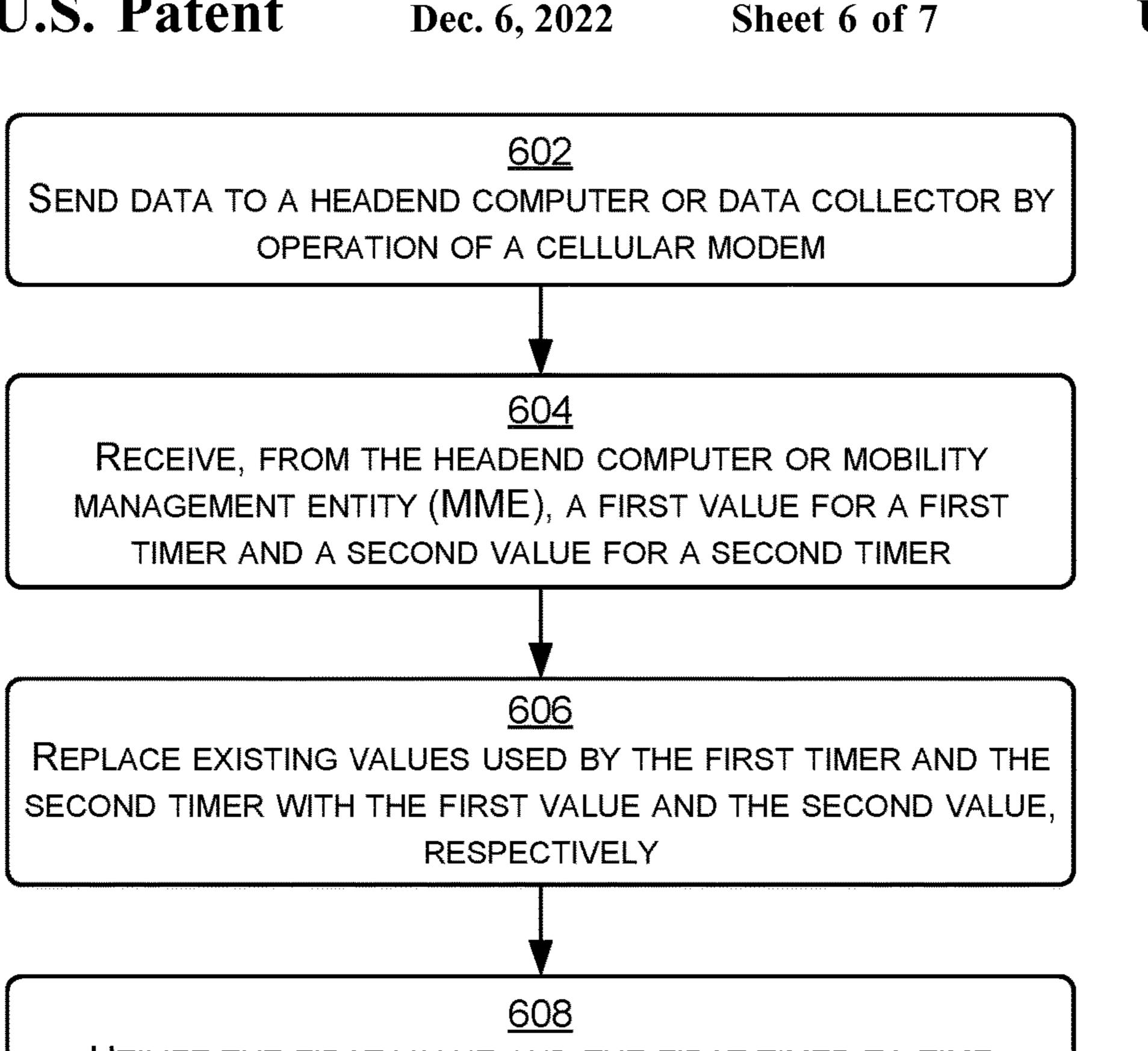
UTILIZE THE FIRST VALUE AND THE FIRST TIMER TO TIME PERIODS DURING WHICH THE CELLULAR MODEM IS IN A POWER-SAVE MODE (PSM)
