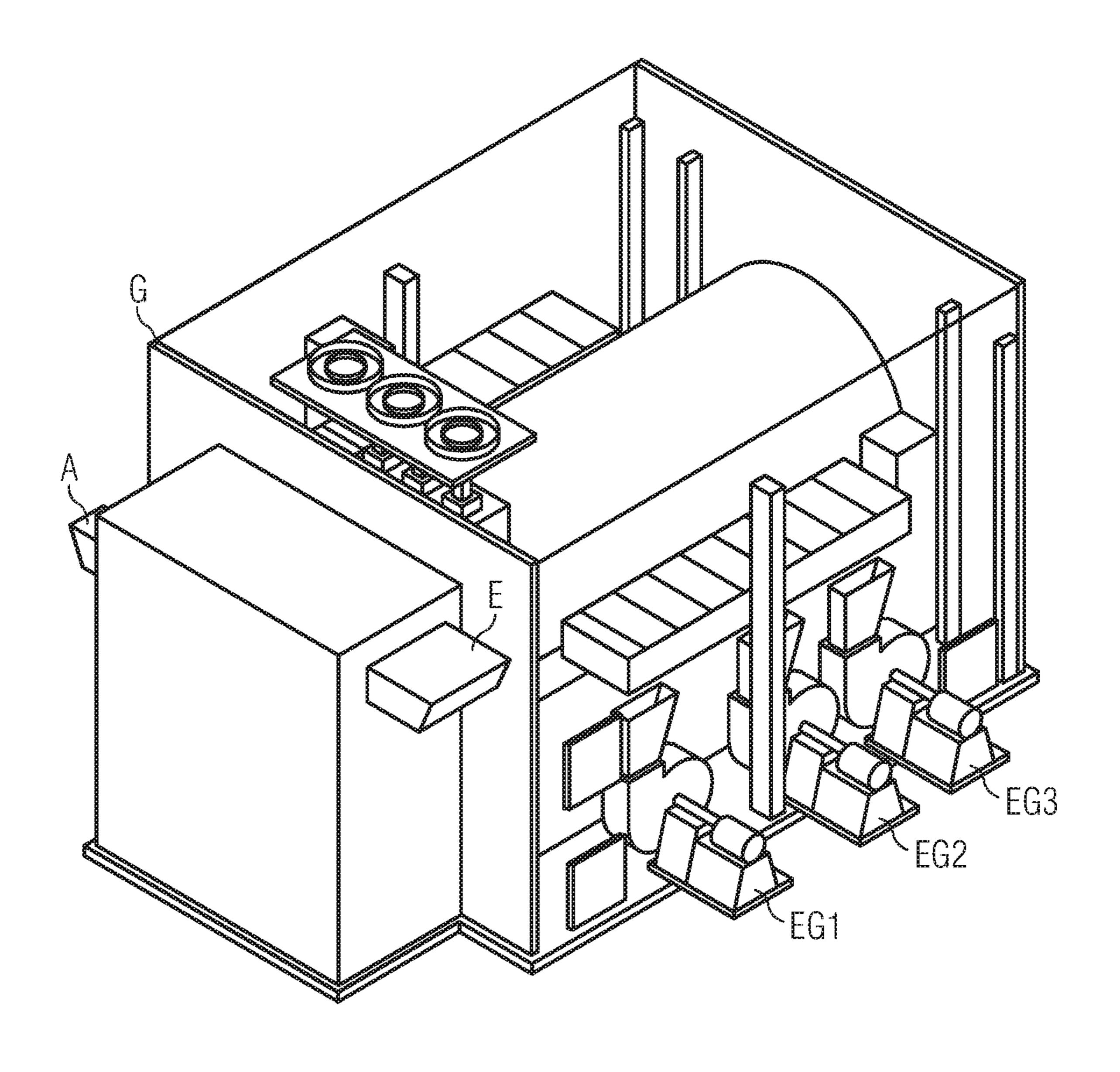
SPEED-REGULATED EXTERNAL FANS FOR THE TEMPERATURE-CONTROLLED THROUGHPUT VENTILATION OF TURBOGENERATORS, PHASE SHIFTERS, AND ROTATING ELECTRICAL MACHINES FOR NETWORK STABILIZATION
