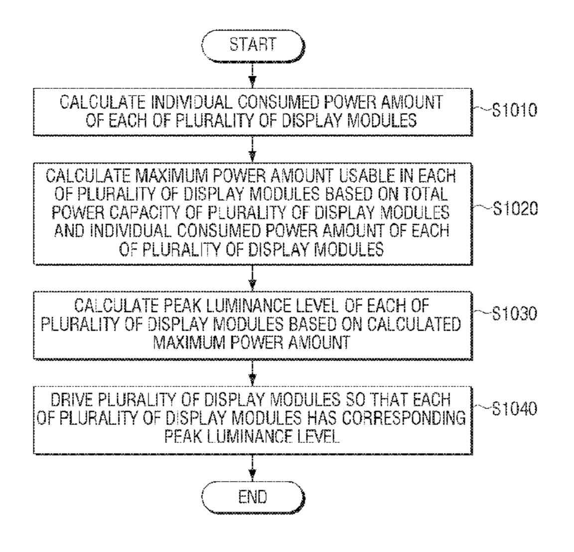
information, the plurality of driving modules such that each of the plurality of display modules has the corresponding peak luminance level.
