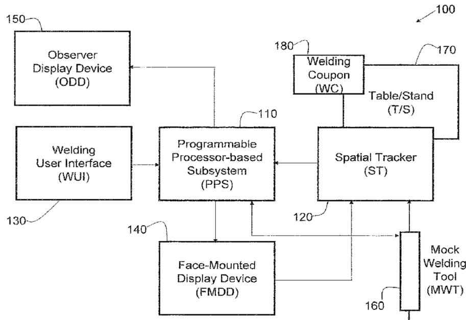
virtual reality welding system and analyzing the data to characterize a student welder's progress and to provide training.
