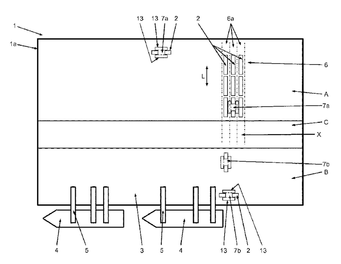
rization to enter the transfer zone in order to travel through the transfer zone. In the absence of granted authorization for entry of a manually guided transport vehicle into a transfer region of the transfer zone, an intervention is automatically implemented in a controller of the transport vehicle in such a way that at least full entry, but optionally even partial entry, to the transfer zone is prevented.
