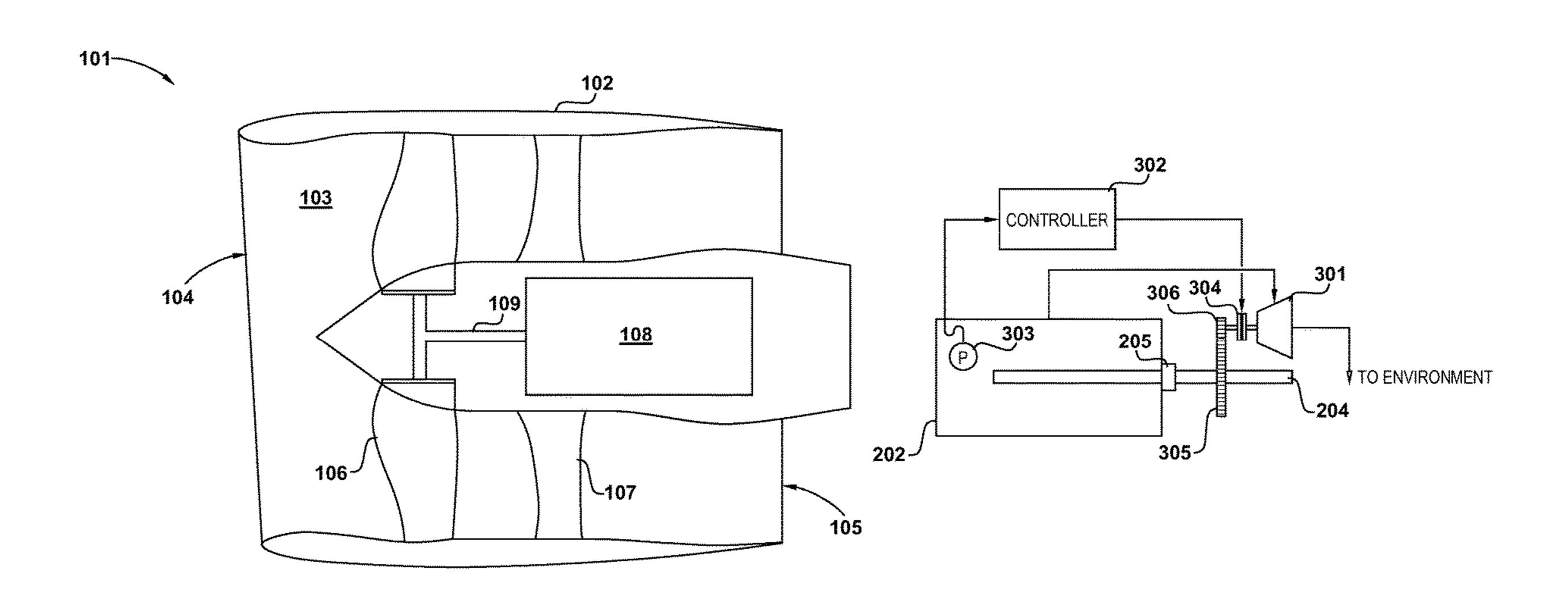
system depressurises the casing below an external pressure to prevent electrical breakdown within gas in the casing of the electric machine.
