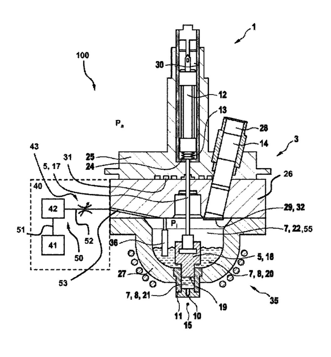
metal (14) can be caused to pass through the outlet opening (10). The invention is distinguished by the fact that the device (40) for generating the inert atmosphere (22) is arranged outside the print head (1), wherein said device comprises an accumulator (41), at least one means (42, 43) for pressure control, and a gas line (50, 51, 52). The invention furthermore relates to methods for operating the device (100).
