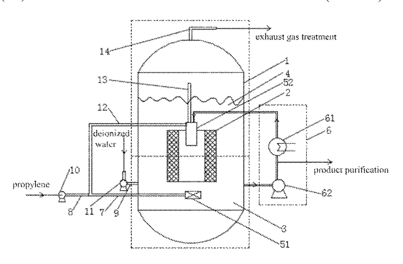
under a lower preset operating condition. The micro-scale bubbles can be fully mixed with the deionized water to from a gas-liquid emulsion. By fully mixing gas and liquid phases, it can ensure that the deionized water in the system is in full contact with propylene, and they are fully in contact with the catalyst, which effectively improves the efficiency of preparing isopropanol.
