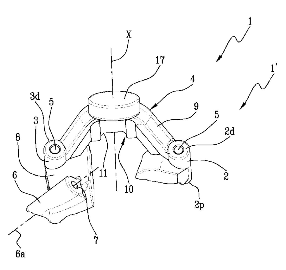
line joining the longitudinal axes of the first and second guide members. The navigation guide also comprises a single additional third guide member that is integral with the frame and is adapted to abut on a second vertebra.
