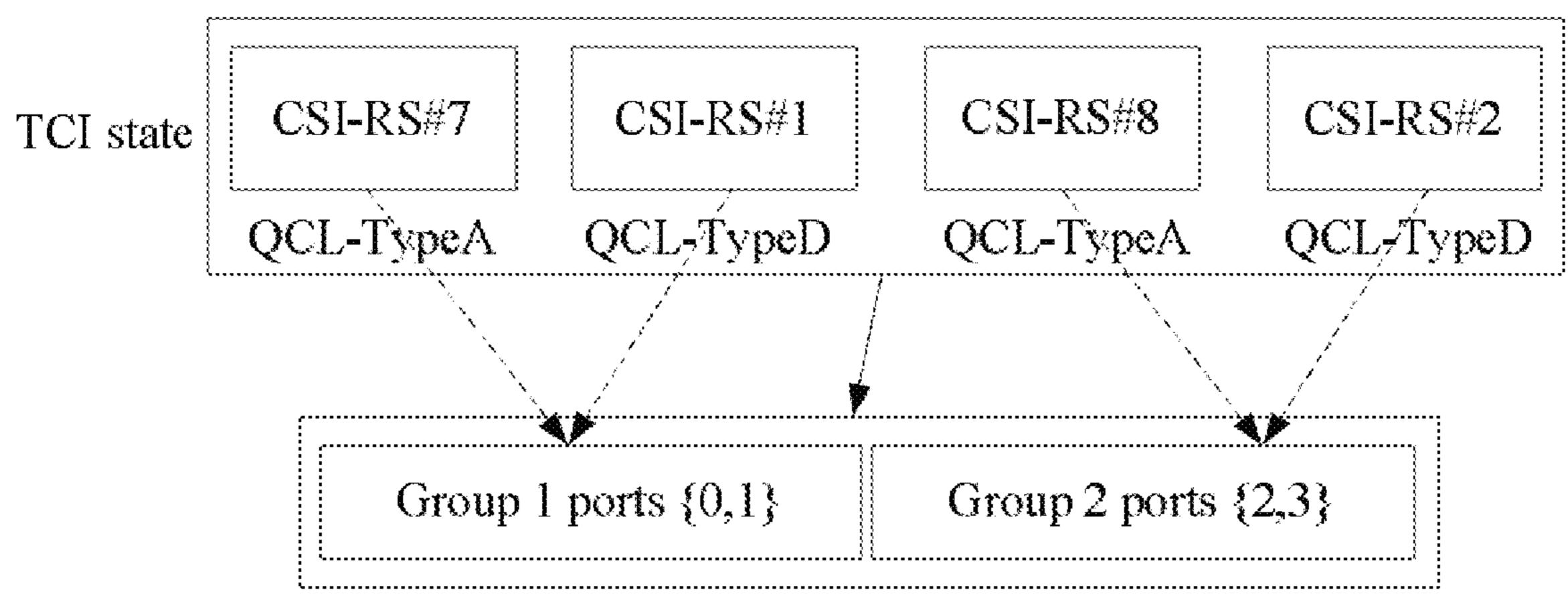
source reference signal, to acquire an extended TCI state; and transmitting the extended TCI state and the target reference signal to a UE, so that the UE determines large-scale parameters of the ports for the target reference signal. TCI configuration of multi-panel, multi-Transmission Reference Point (TRP) and multi-beam communication is supported.
