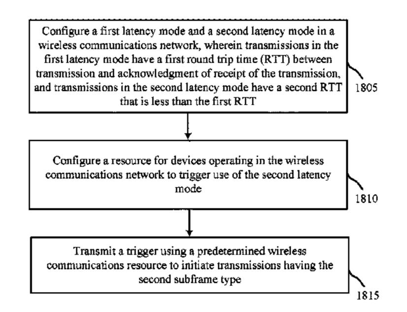
duration and the second subframe type comprising symbols of a second duration that is shorter than the first duration. Communications may be initiated by transmitting a trigger from the UE or eNB using the dedicated resource, and initiating communications following the trigger. The duration of time between the trigger and initiating communications can be significantly shorter than the time to initiate communications using legacy LTE communications.
