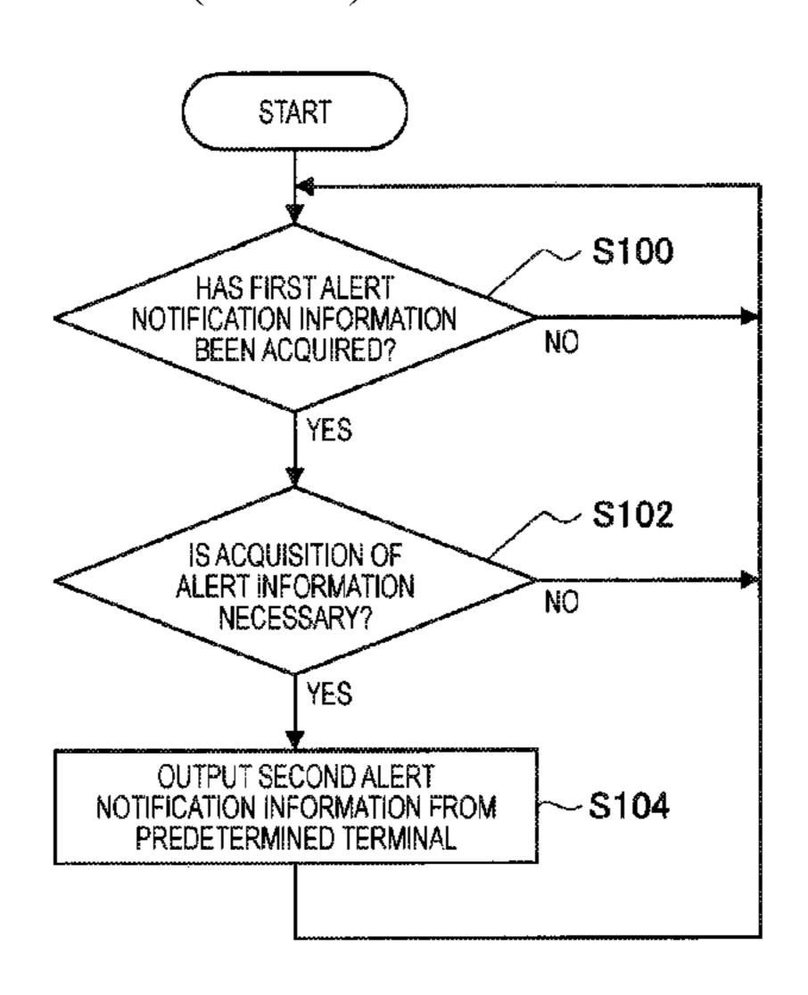
processing unit configured to output second alert notification information corresponding to the operation mode from a predetermined terminal to which a processing circuit having a function to acquire the alert information is electrically connected, in a case where acquisition of the alert information is determined to be necessary.
