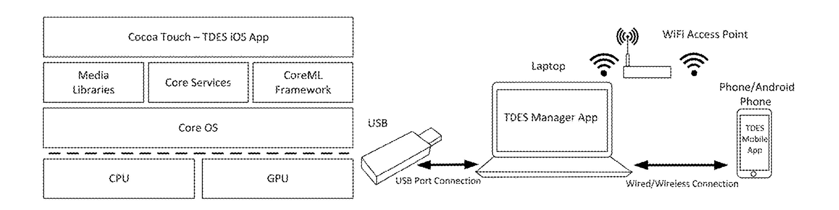
tation of such a targeted data extraction system (TDES) for mobile devices. The TDES assumes consent of the user and implements state of the art filtering using machine learning techniques. This system can be used to identify and extract selected data from smart phones, in real time at the scene of the crime.
