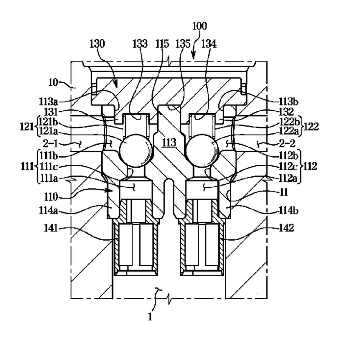
passage and opened and closed by the hydraulic pressure of the fluid; and a stopper member press-fitted to the valve housing.
