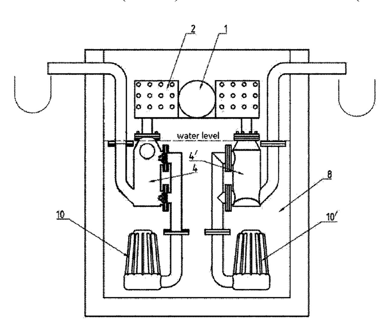
reverse flow of wastewater from the pump into the separation chamber to a discharge pipe. A solid particles separator arranged between the separation chamber and the bidirectional pipe separates solid particles contained in wastewater in the separation chamber.
