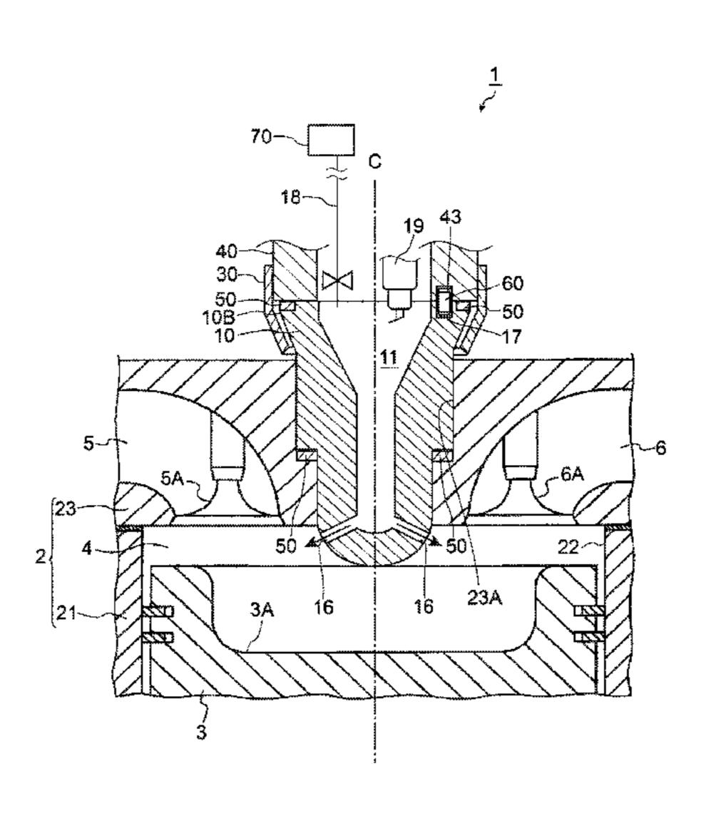
between the precombustion chamber cap holding member and the proximal end portion when the precombustion chamber cap holding member suspends and supports the precombustion chamber cap.
