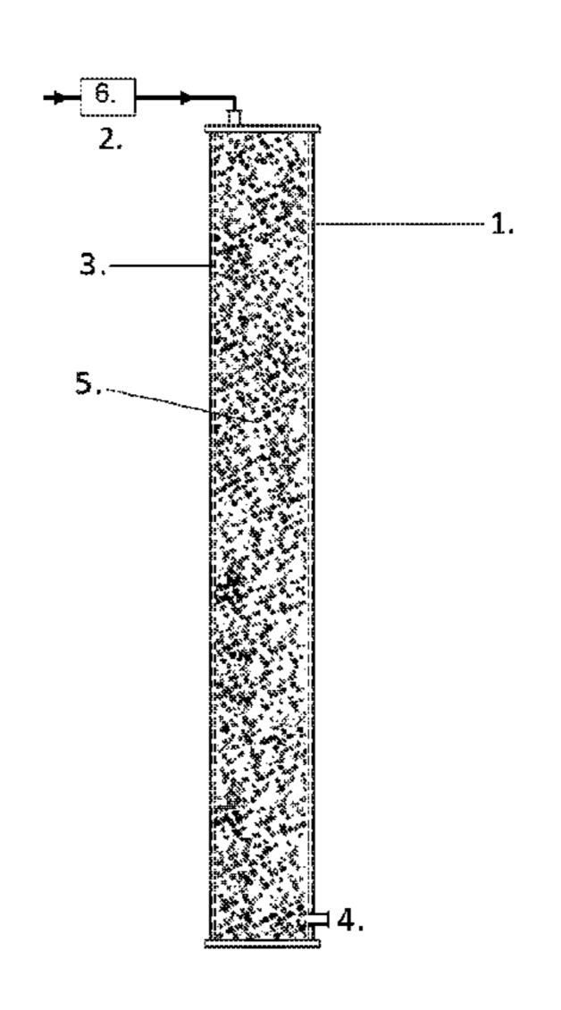
20% to 60% of the volume of the bioreactor, and the liquid phase is at least 20% of the reactor volume, The unsaturated capillary conductivity of filling/packing solid material of the bioreactor is at least 0.1 cm/h. The solid state fermentation bioreactor enables a large gas-liquid interface, in which the filling material has a good capillary conductivity despite the unsaturated state.
