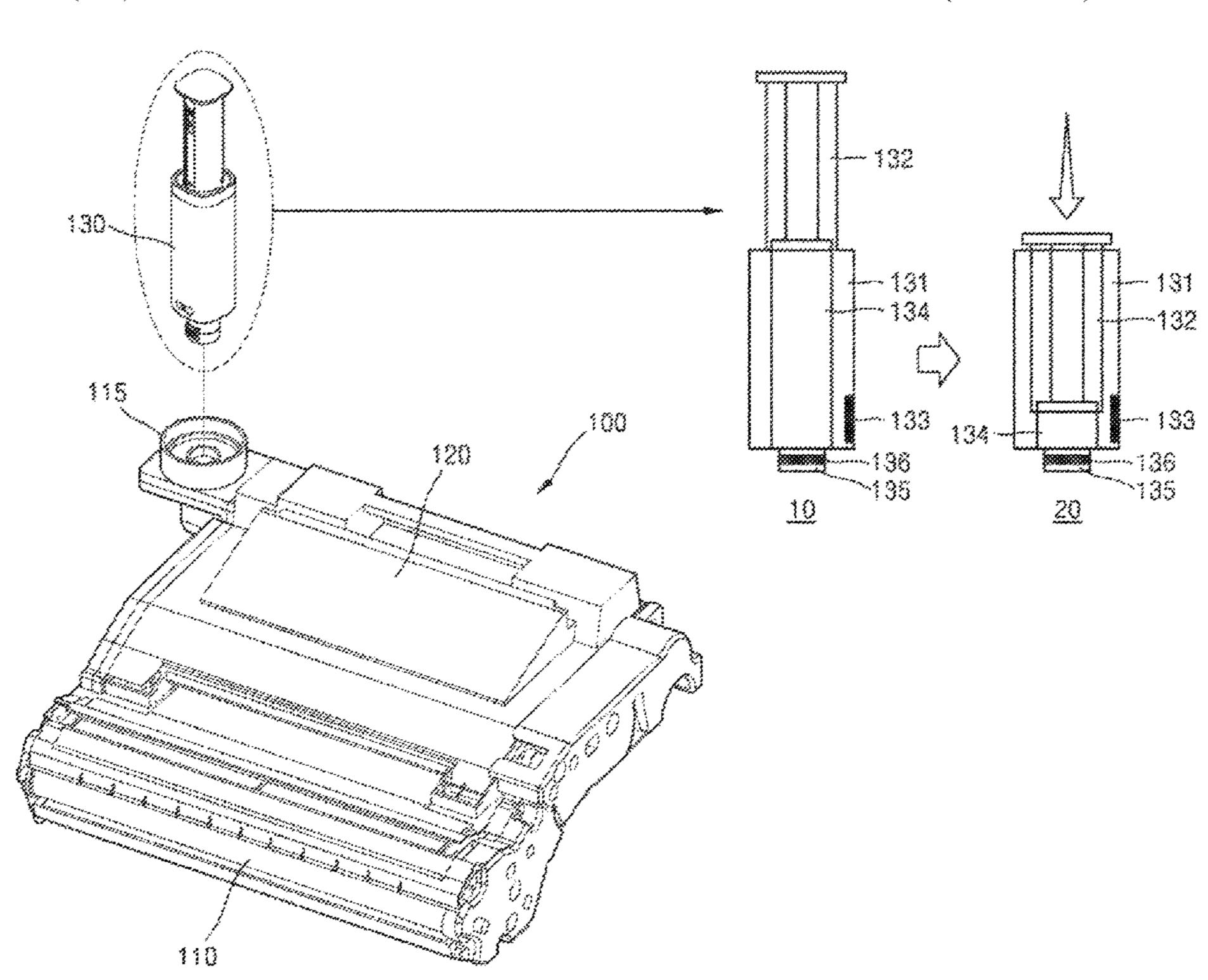
cartridge in the image forming apparatus, based on completion of injecting toner from the TRK into the cartridge, controlling the TRK to store information indicating a toner refill completion in a memory of the TRK and updating information of an amount of remaining toner of the cartridge based on an amount of the toner injected into the cartridge from the TRK.
