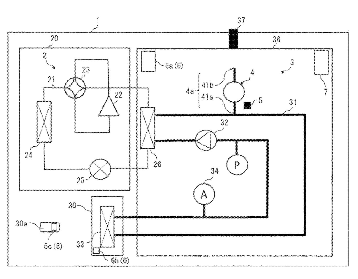
controller activates the notification device depending on the concentration of the refrigerant detected.
