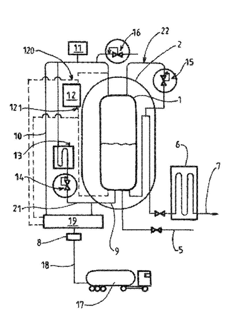
filling pipes, wherein the tank comprises a sensor assembly which measures the pressure in the first casing, said distribution valve assembly being configured to automatically adjust the pressure in the first casing, during filling, to a predetermined pressure setpoint (Pc) by means of the automatic distribution of the flow rate of fluid from the source in the filling pipes, depending on the pressure setpoint (Pc) and the pressure measured by the sensor assembly.
