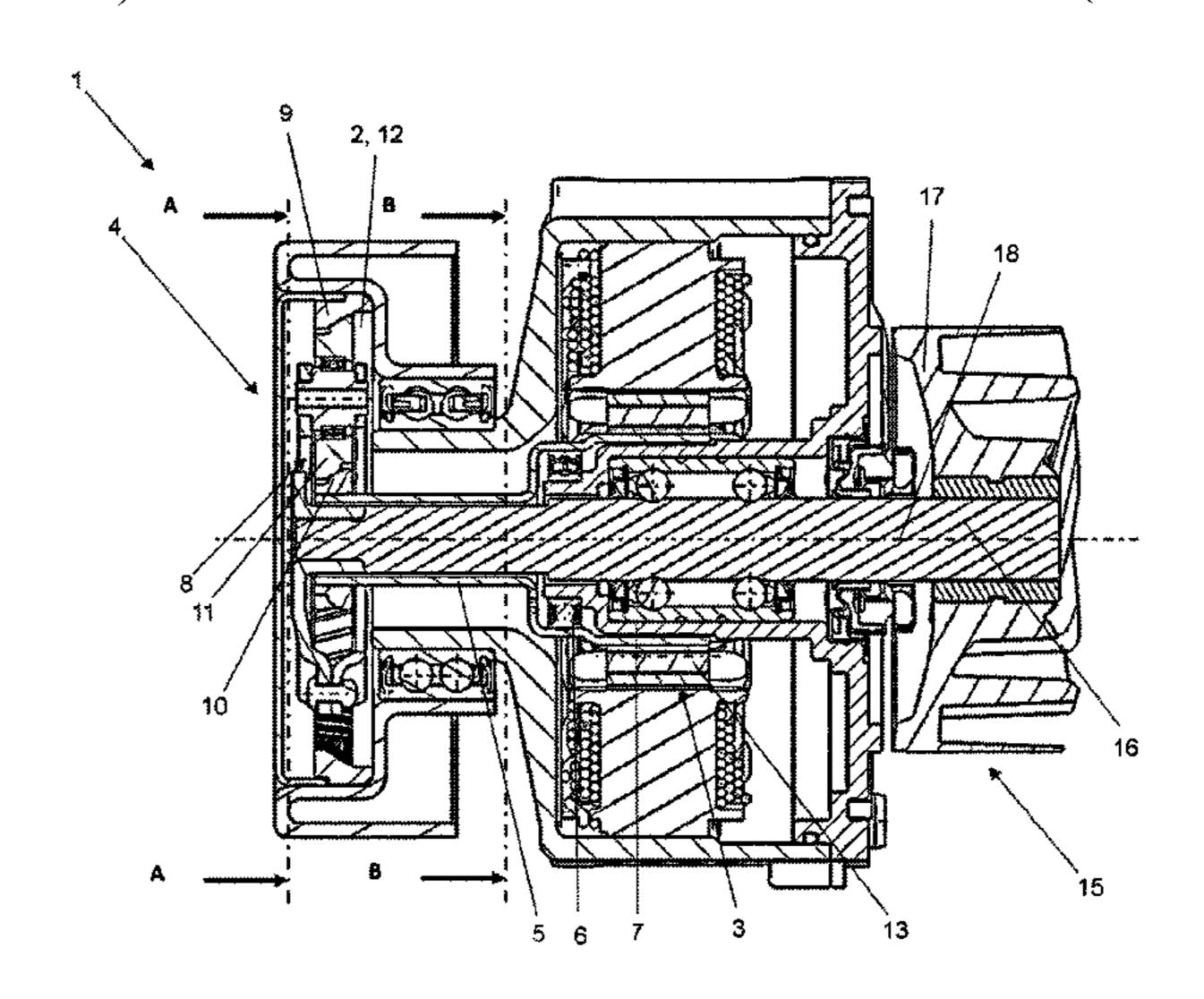
mounted at one side on a housing of the pump assembly via a ball bearing and at the other side in a gear stage of the planetary gearbox.
