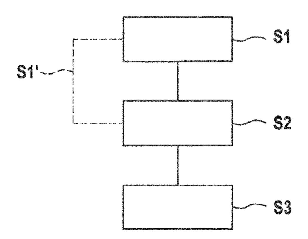
S1 MULTIPLE SUCCESSIVE INSTANCES OF ACTUATION OF THE LOCKING DEVICE S1' GENERATE FURTHER SIGNAL SEQUENCE S2 COMPARING CHRONOLOGICAL SIGNAL SEQUENCE S3 RELEASING THE CAR FOR DRIVING OPERATION
