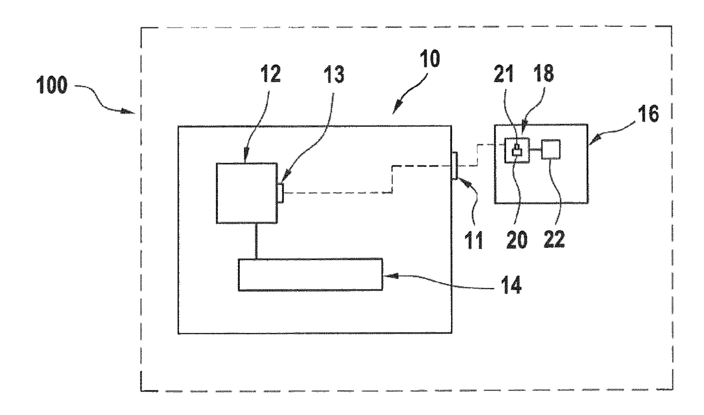
10 CONTROL UNIT 11 INTERFACE 12 CONTROLLER 13 INTERFACE 14 MEMORY DEVICE 16 SHAFT DOOR 18 LOCKING DEVICE 20 SENSOR ELEMENT 21 SWITCH 22 LOCK 100 ELEVATOR INSTALLATION
