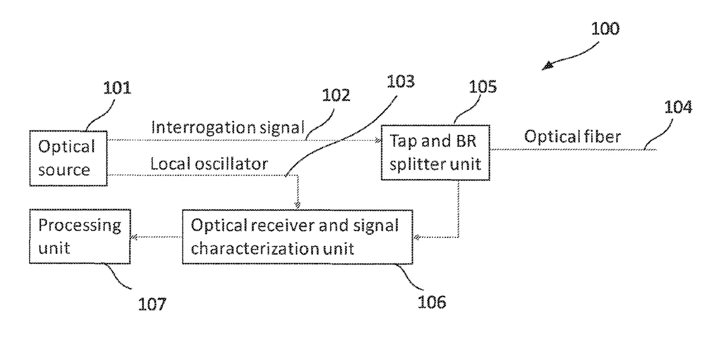
the measurement result such that an effect of fluctuations in the interrogation phasor on the measured response from the fiber is reduced; and applying distributed back-reflection processing to the receiver output signal. Finally, the method comprises extracting the response from the optical fiber from the distributed back-reflection processing output. A system for measuring a response from an optical fiber providing distributed back reflections is also disclosed.
