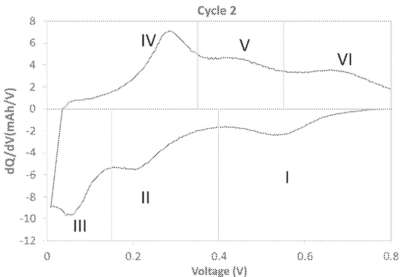
Figure 3. Differential capacity vs voltage plot for Silicon-Carbon Composite 3 from 2<sup>nd</sup> cycle to 5<sup>th</sup> cycle using a half-cell.
