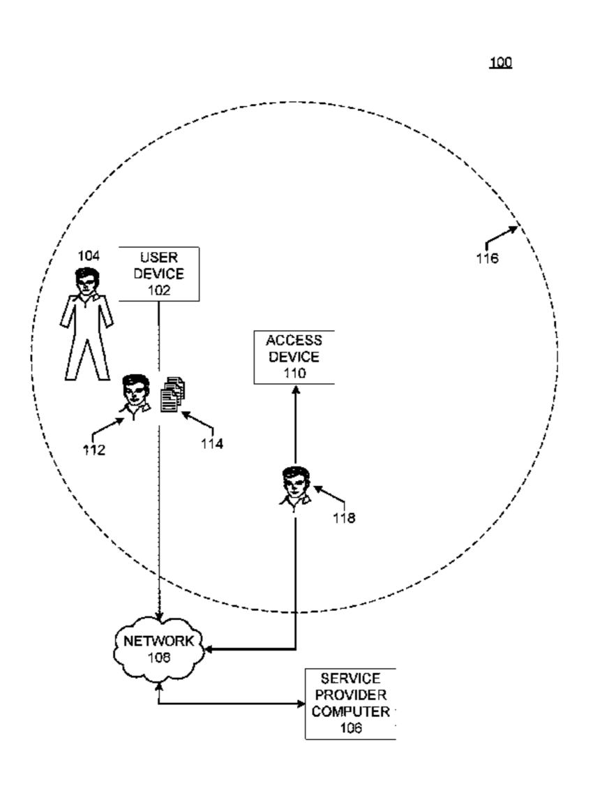
system may provide the access device with account information stored in relation to the matched biometric template. The access device may then complete a transaction using the provided account information and grant access to the requested resource.
