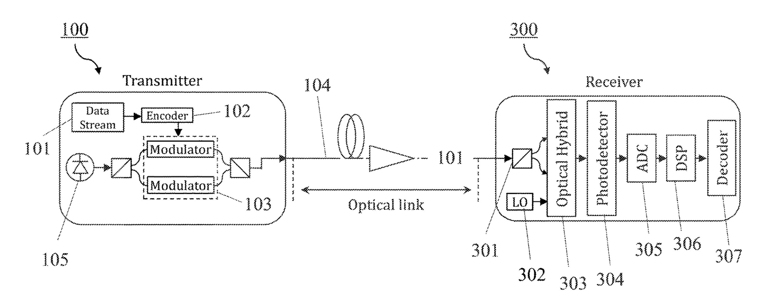
consecutive transmission time slots to modulate two carrier waves, and to transmit the two carrier waves over the orthogonal polarizations of the optical carrier. The set of constellation points do not include any constellation point with parallel Stokes vectors in the two consecutive transmission time slots but comprise constellation points with orthogonal Stokes vectors.
