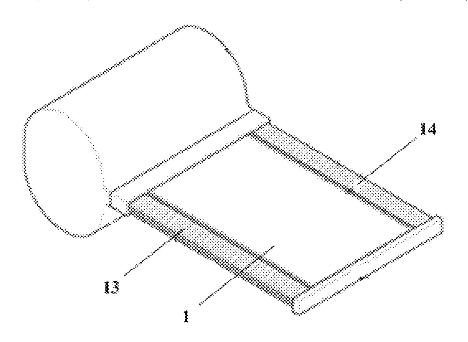
supporting components comprises: a first supporting component and a second supporting component which are opposite to each other. A first end of the first supporting component is fixedly connected to a first end of the rotating component, and a second end of the first supporting component is fixedly connected to a first end of the second fixing part at the second side of the display panel.
