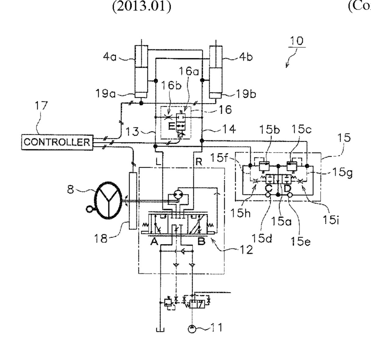
between the feed line and the return line. The controller opens the electromagnetic valve in response to an oil pressure in the feed line.
