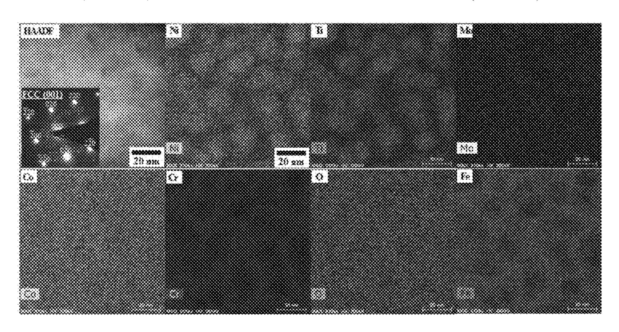
In the present invention, the alloy member having a chemical composition comprising elements of Co, Cr, Fe, Ni, and Ti each in an amount within a range of 5 atomic % or more and 35 atomic % or less and Mo in an amount within a range of more than 0 atomic % and 8 atomic % or less, the reminder consisting of unavoidable impurities, wherein ultrafine grains having an average grain diameter of 100 nm or less are dispersed and precipitated in a parent phase crystal.
