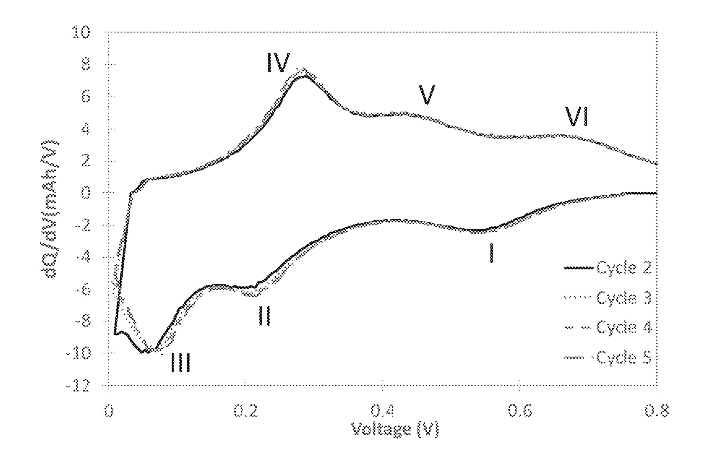
Figure 4. dQ/dV vs V plot for various silicon-carbon composite materials.
