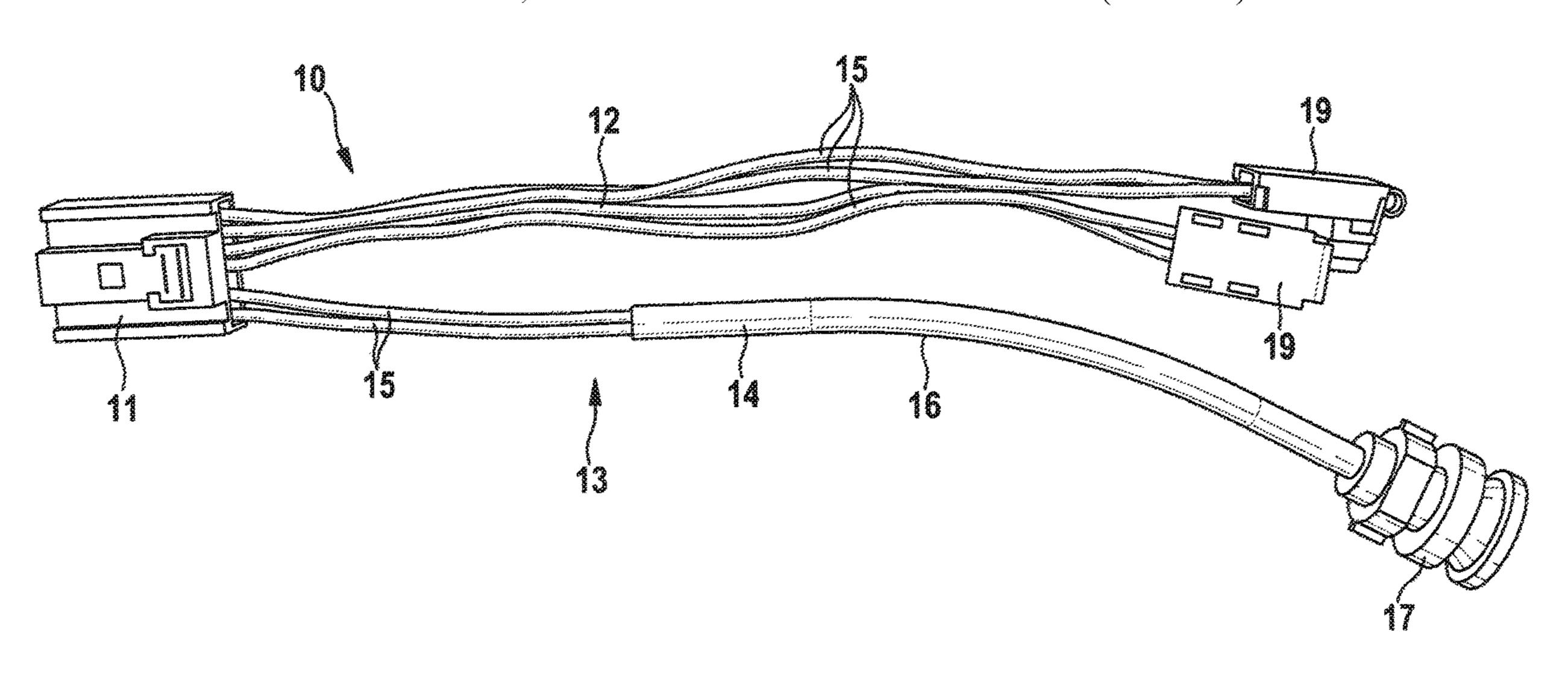
tor (11) for connecting the connector (11) to a vehicle wiring harness, and at least one actuator unit (13) having a pyrotechnic actuator (17) and an actuator connecting cable (14) which is formed integrally with the actuator unit (13) and is connected to the connector (11). The invention further relates to an airbag module, vehicle cabling and a vehicle occupant safety system having a wiring harness of this kind and to a method of production.
