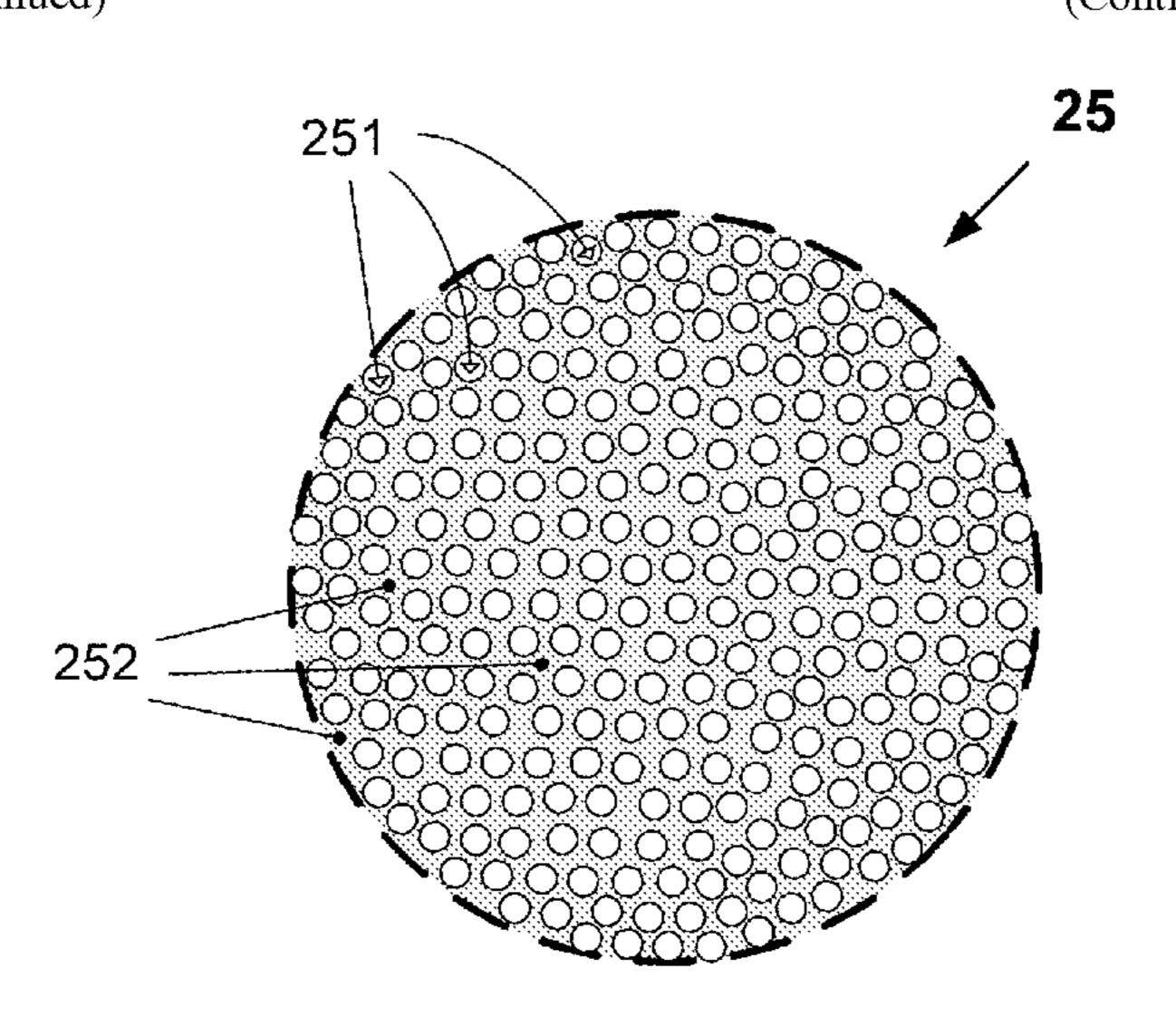
monofilament, measured at 23° C., is greater than 35 GPa. The real part of the complex modulus of the monofilament, measured at 190° C. by the DMTA method, is greater than 30 GPa. Pneumatic or non-pneumatic tires are reinforced with such a composite monofilament.
