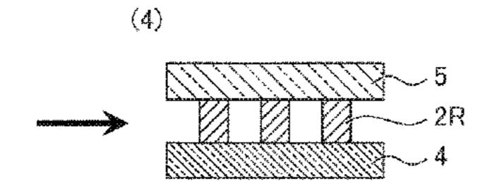
first substrate, and pressure-bonding the first substrate, the photoresist pattern, and the second substrate.
