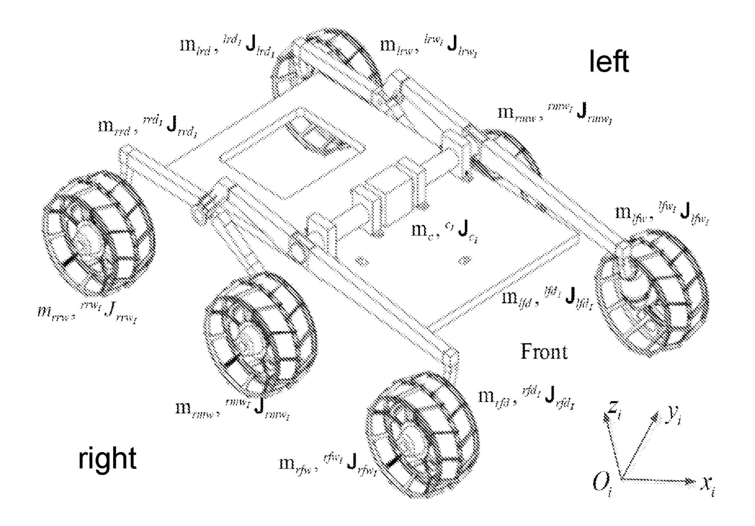
$^{O_l}$  — the origin of axis  $^l$   $m_l$  — the mass of axis  $^l$
