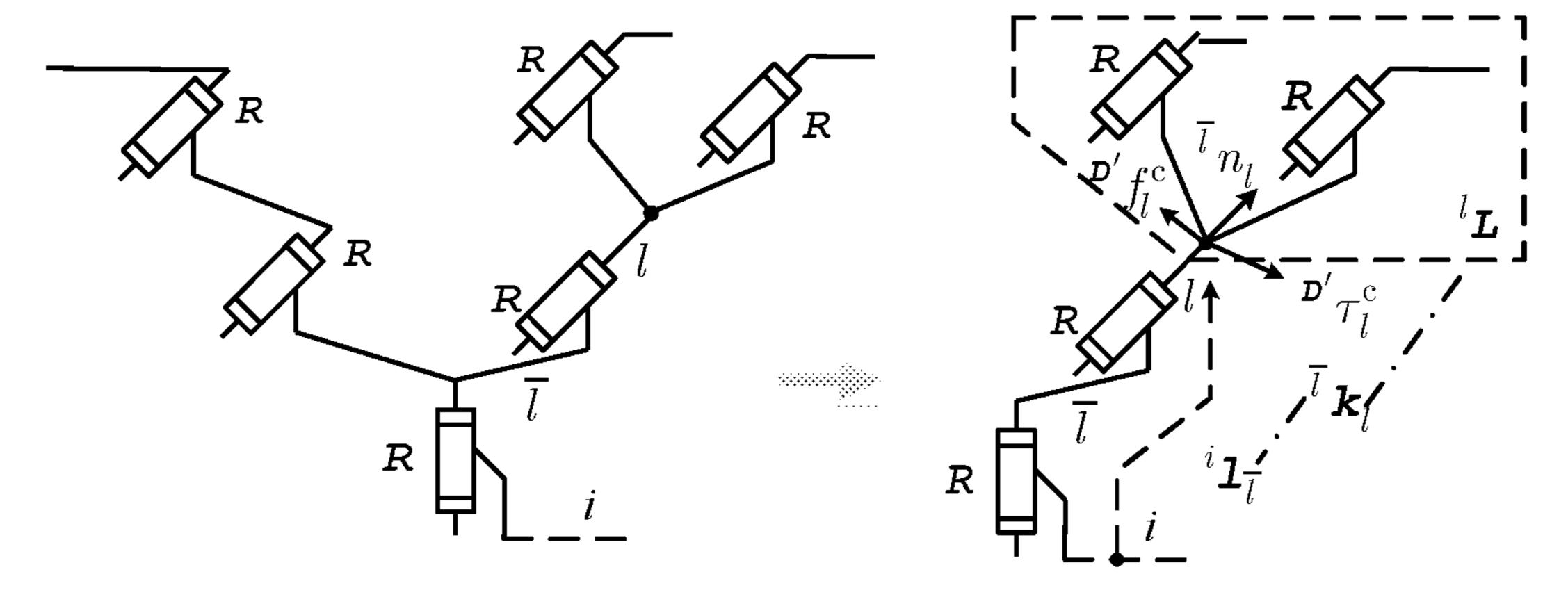
${}^{i}\mathbf{k}_{\overline{l}}$  — the kinematic chain of the axis  $\overline{l}$
