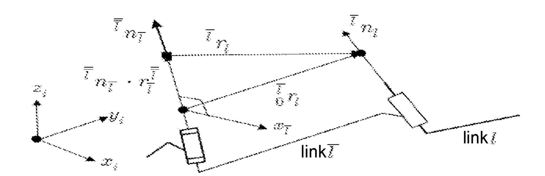
$^{\overline{\overline{l}}}n_{\overline{l}}$  — the axis-invariant
