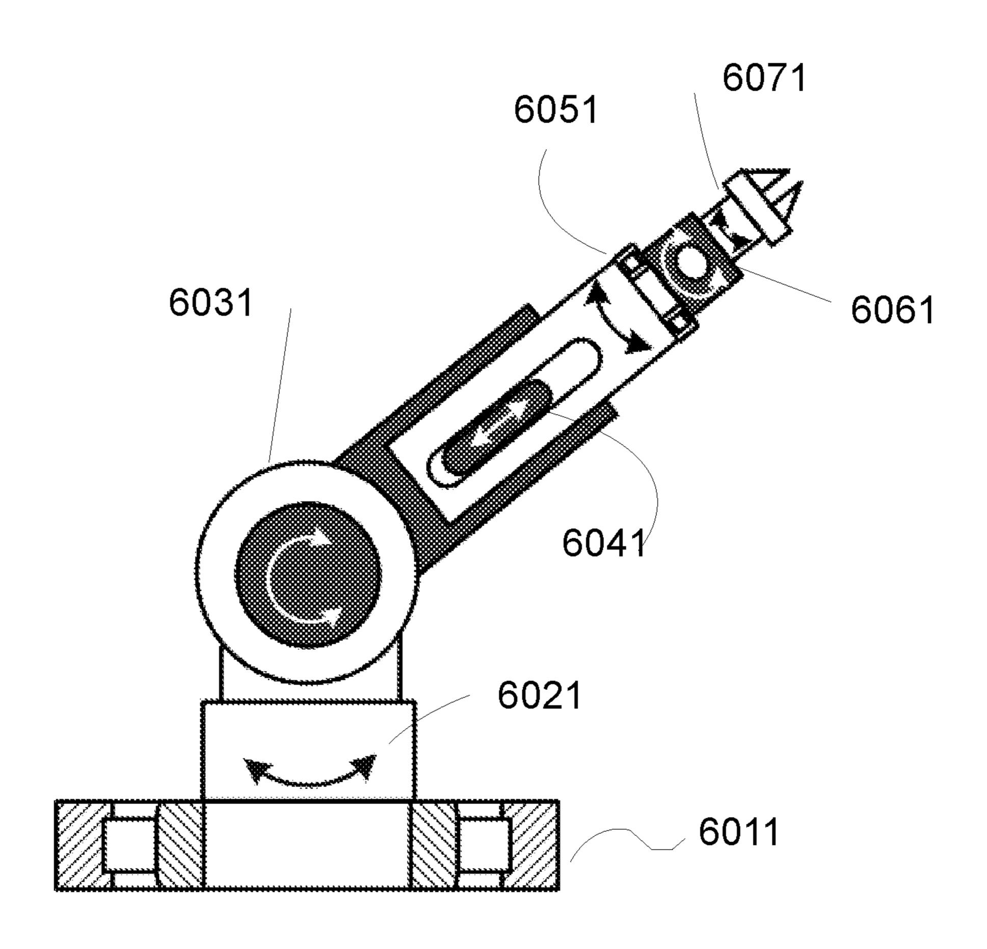
6011 — base 6021 — the first link and revolute joint pair  ${}^{0}R_{1}$ 6031 — the second link and revolute joint pair  ${}^{1}\mathbf{R}_{2}$  6041 — the third link and revolute joint pair  ${}^{2}\mathbf{R}_{3}$ 6051 — the first gripper and revolute joint pair  ${}^3\mathbf{R}_4$ 6061 — the second gripper and revolute joint pair  ${}^4R_5$  6071 — the third gripper and revolute joint pair  ${}^5R_6$
