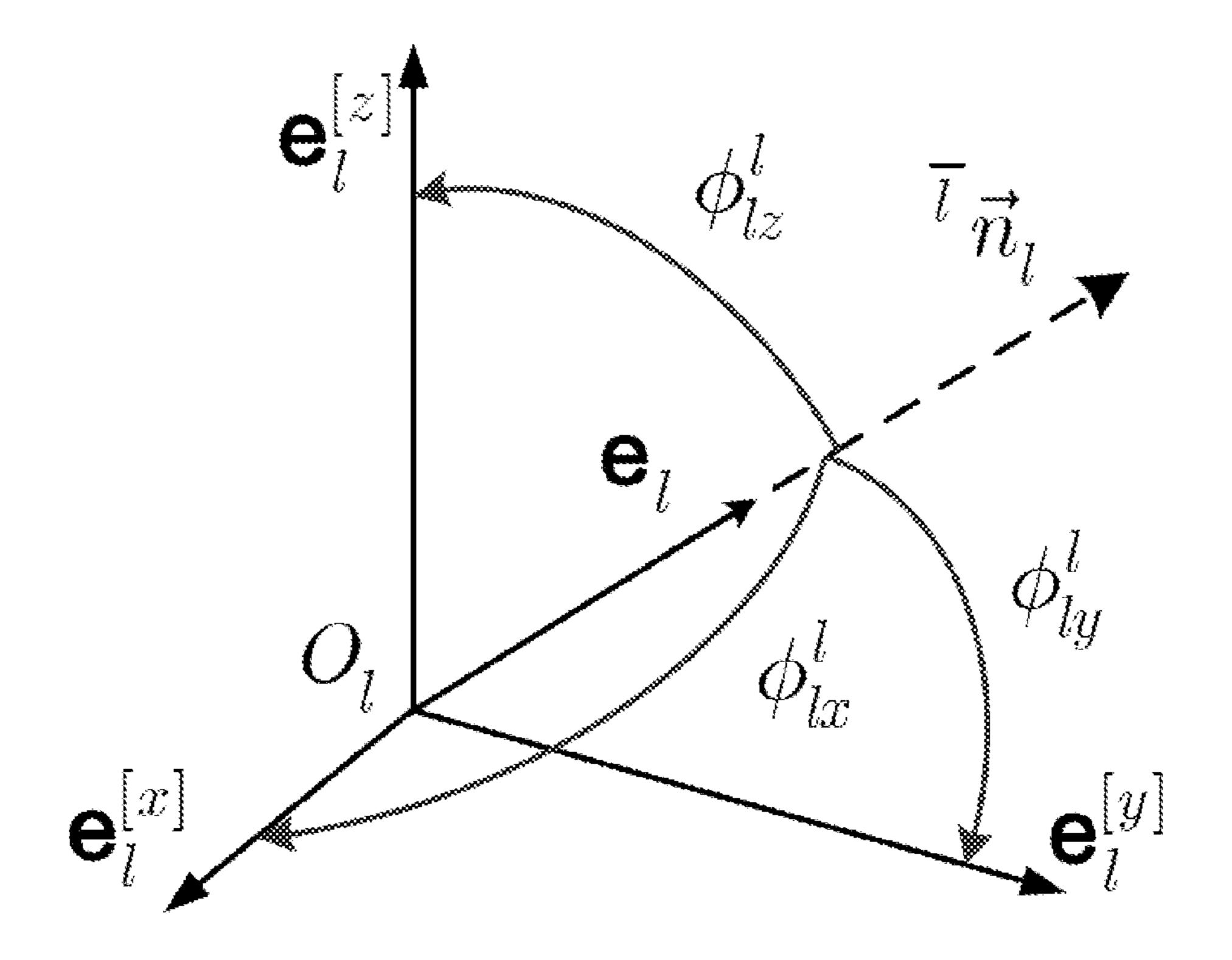
$O_l$  — the origin  $egin{array}{c} oldsymbol{\Theta}_l & - ext{ the basic vector} \\ \hline {}^l ec{n}_l & - ext{ the unit Axis-Vector} \\ \phi^l_{lx} \ , \ \phi^l_{ly} \ , \ \phi^l_{lz} & - ext{ three basic component} \end{array}$
