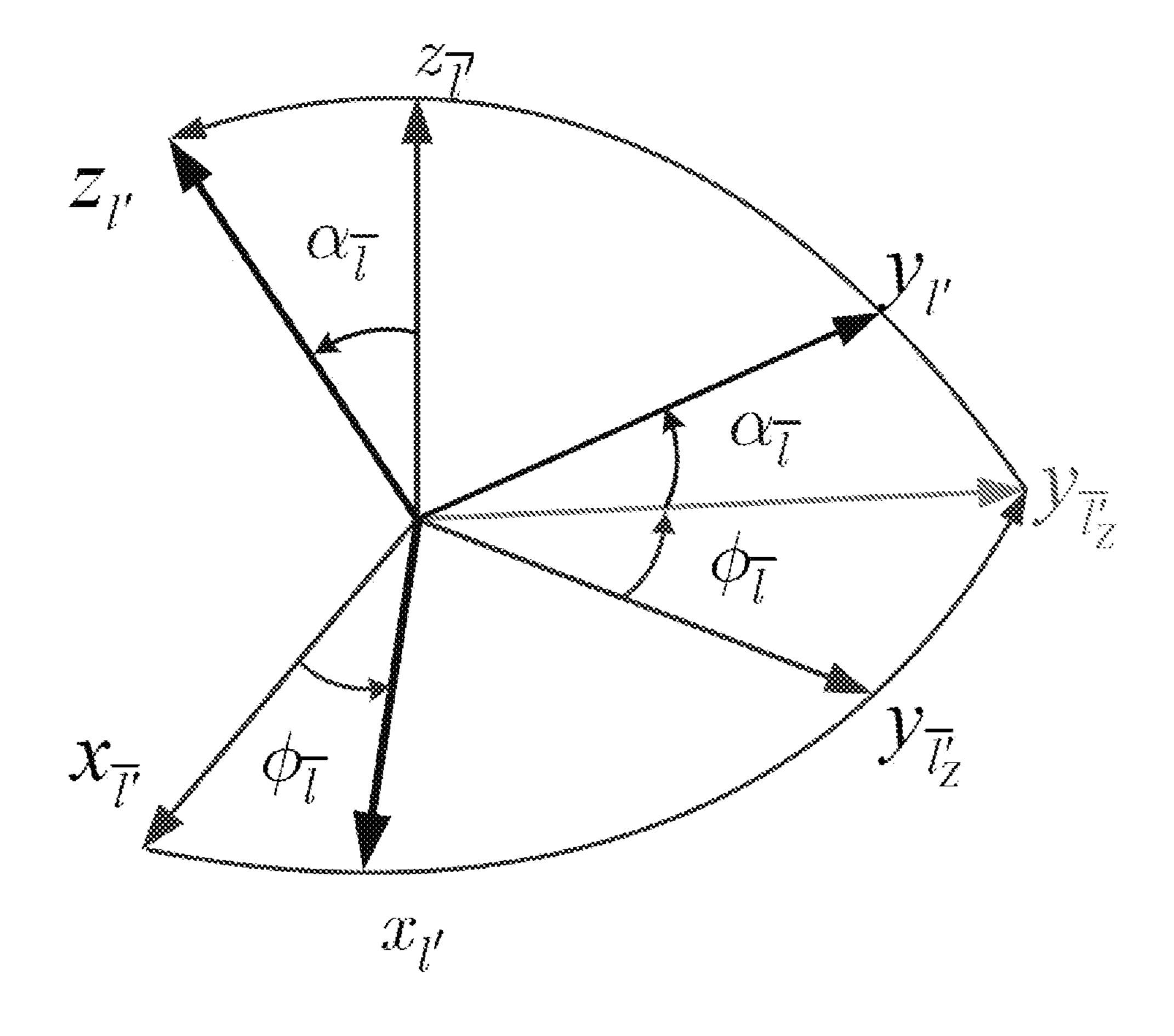
$\phi_{\overline{l}}$  — the rotation angle to the axis  $z_{\overline{l}'}$
