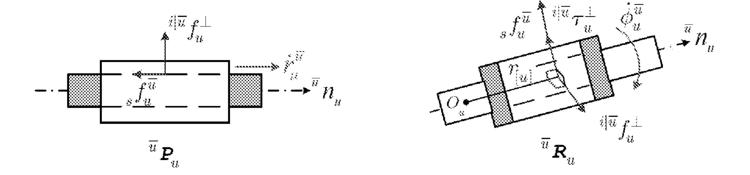
$f_u^\perp$  ,  $\tau_u^\perp$  — the radial constraint force and torque of the Motion-Axis u  $_sf_u^{\overline{u}}$  ,  $_s\tau_u^{\overline{u}}$  — the internal friction force and torque of the Motion-Axis u  $_cf_u^{\overline{u}}$  ,  $_c\tau_u^{\overline{u}}$  — the viscous force and torque of the Motion-Axis u
