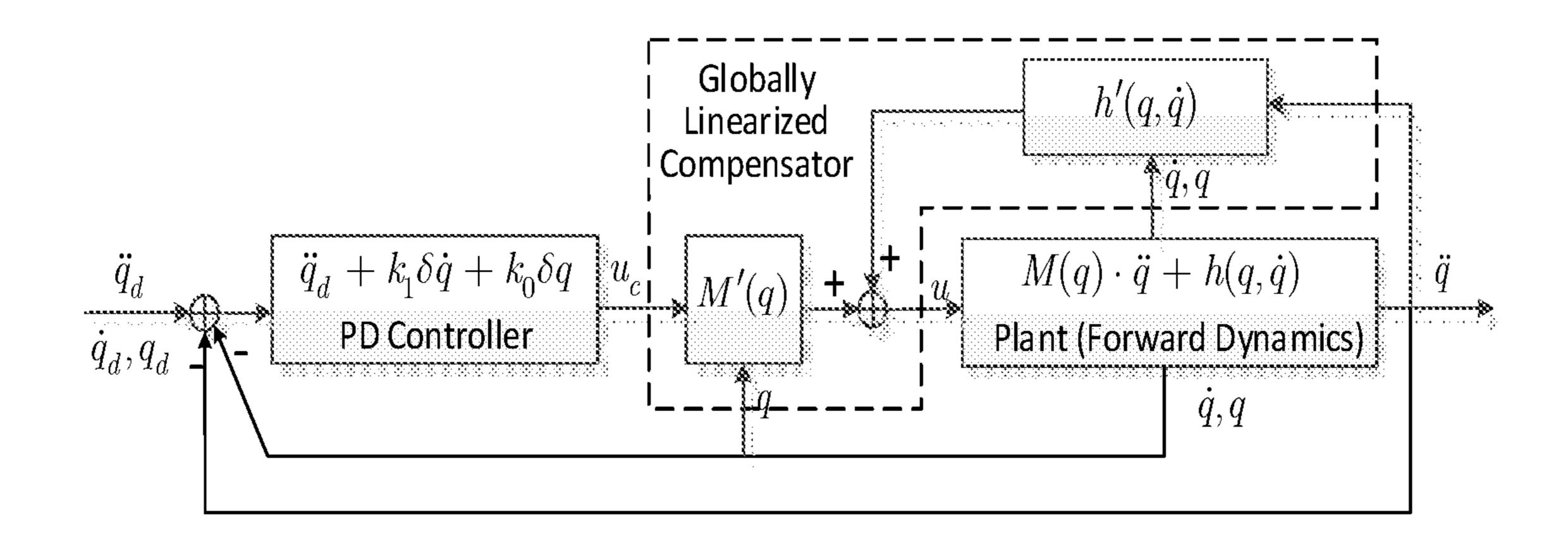
$[\ddot{q}_d, \dot{q}_d, q_d]$  — the disired state  $[\ddot{q}, \dot{q}, q]$  — the achievable state M'(q) — nominal model of M(q)  $h'(q, \dot{q})$  — nominal model of  $h(q, \dot{q})$   $u_f$  — disturbance
