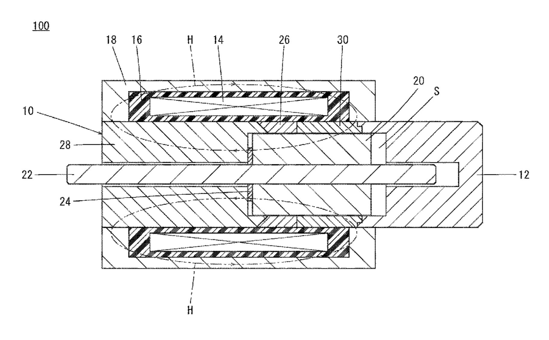
second bonding portion are removed. Thereafter, the non-magnetic member becomes a non-magnetic body, the first magnetic member becomes a first magnetic body, the second magnetic member becomes a second magnetic body and a sleeve is obtained.
