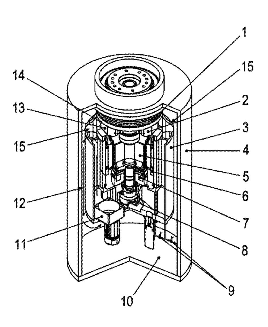
lating airflow is able to be provided within the housing, the recesses in particular guiding the airflow through in the axial direction, and the airflow being returned in the opposite direction in the set-apart region between the stator housing part and the housing.
