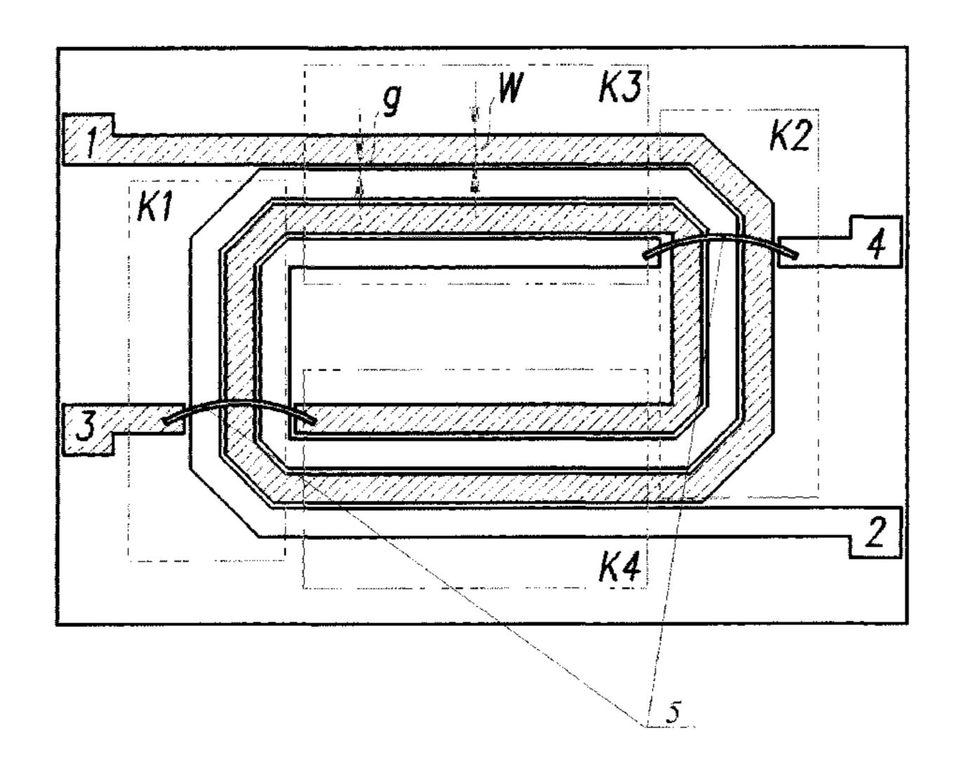
coupler rotated relative to the other around their common center, while clearances between the coupled transmission lines and their cross-sectional dimensions are constant.
