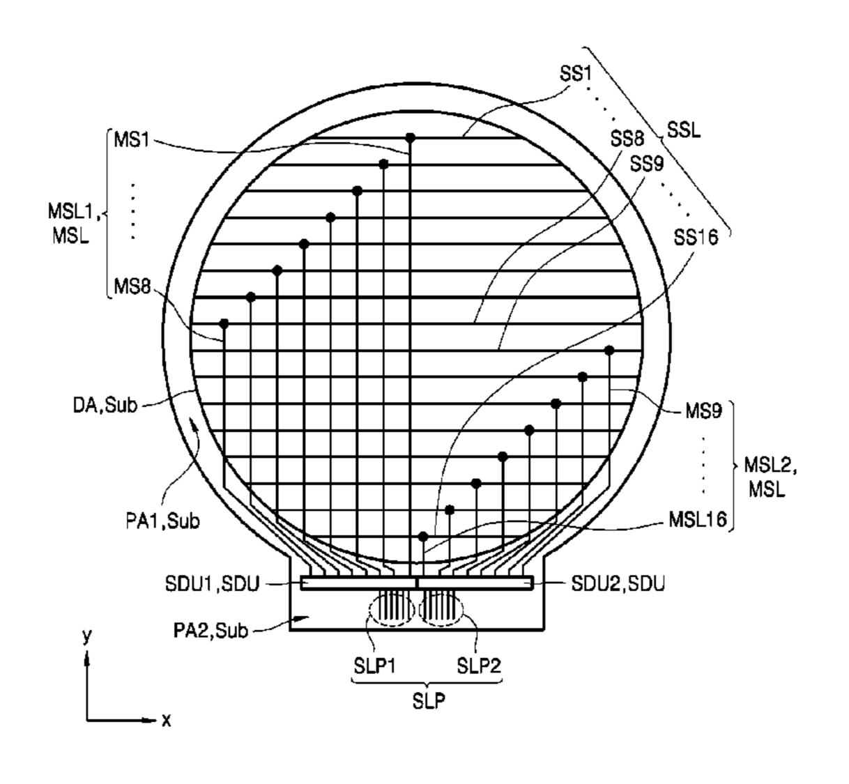
data lines, and scan line pads connected to the main scan lines, the first data line pads, the scan line pads, and the second data line pads being adjacent.
