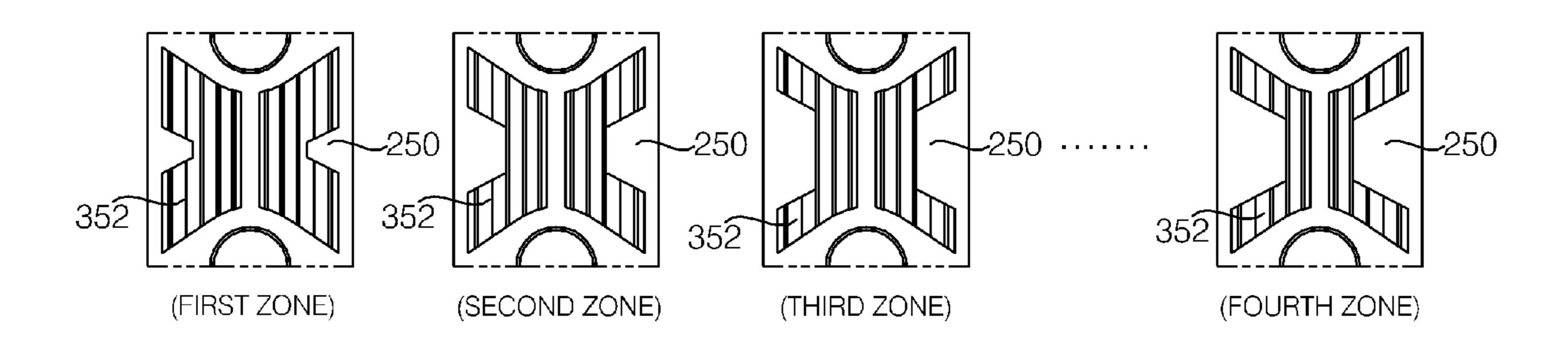
an area LA1 of the louver fin in the first zone is formed to be larger than an area LA2 of the louver fin in the second zone.
