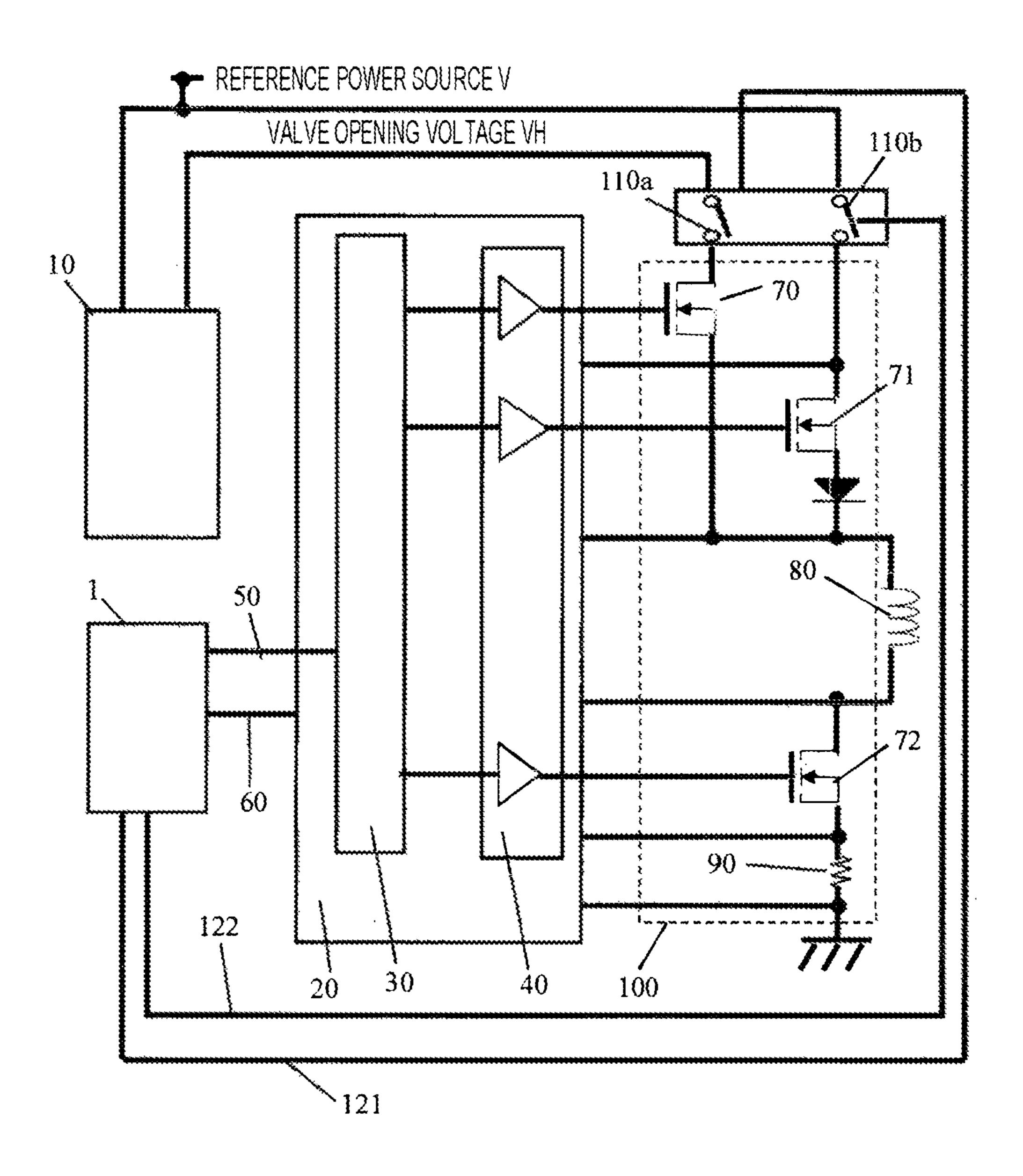
121: CURRENT CUTOFF MECHANISM CONTROL SIGNAL LINE A 122: CURRENT CUTOFF MECHANISM CONTROL SIGNAL LINE B
