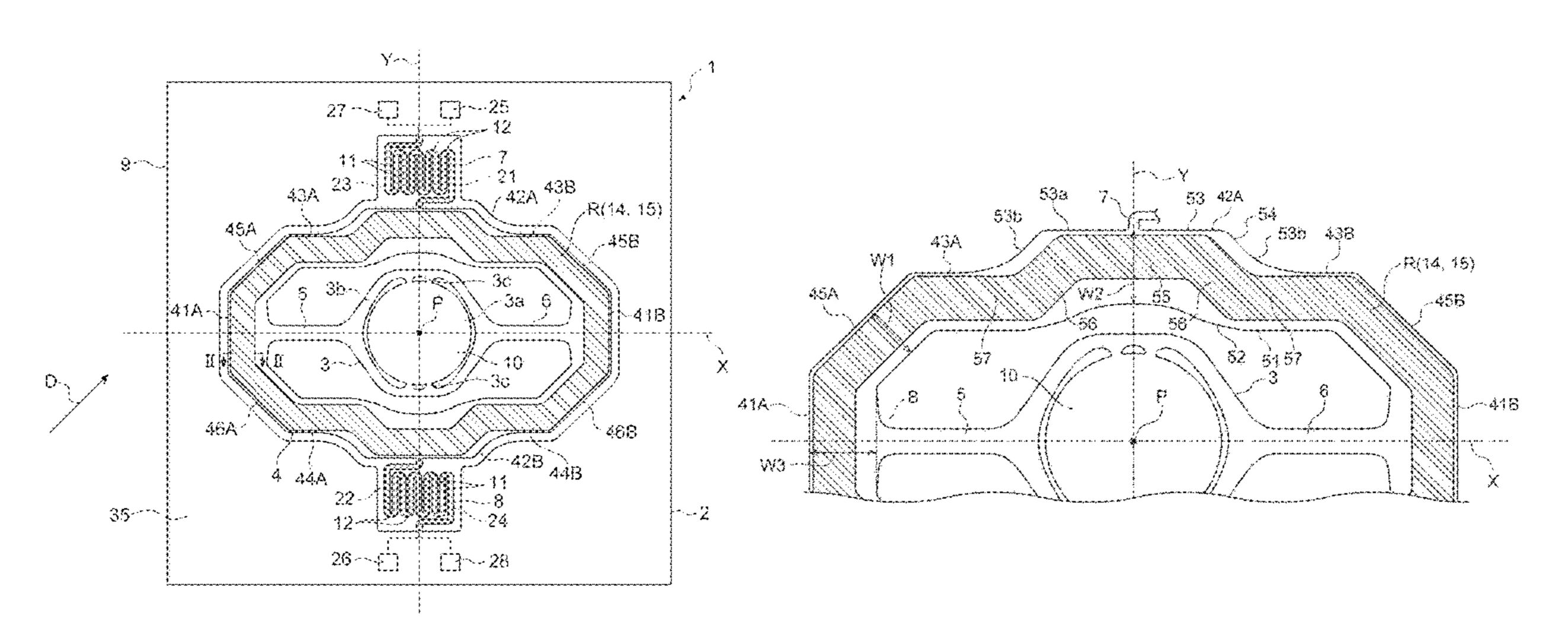
of the second connection portions, includes a depression recessed in a second axis direction, and an outer edge of each of the pair of second connection portions, includes a protrusion protruding in the second axis direction.
