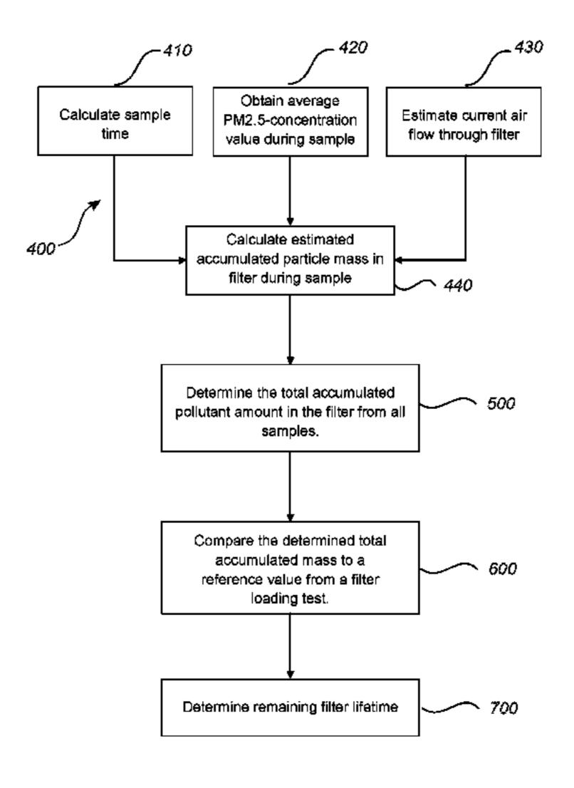
volume is estimated based on a current air flow through the filter.
