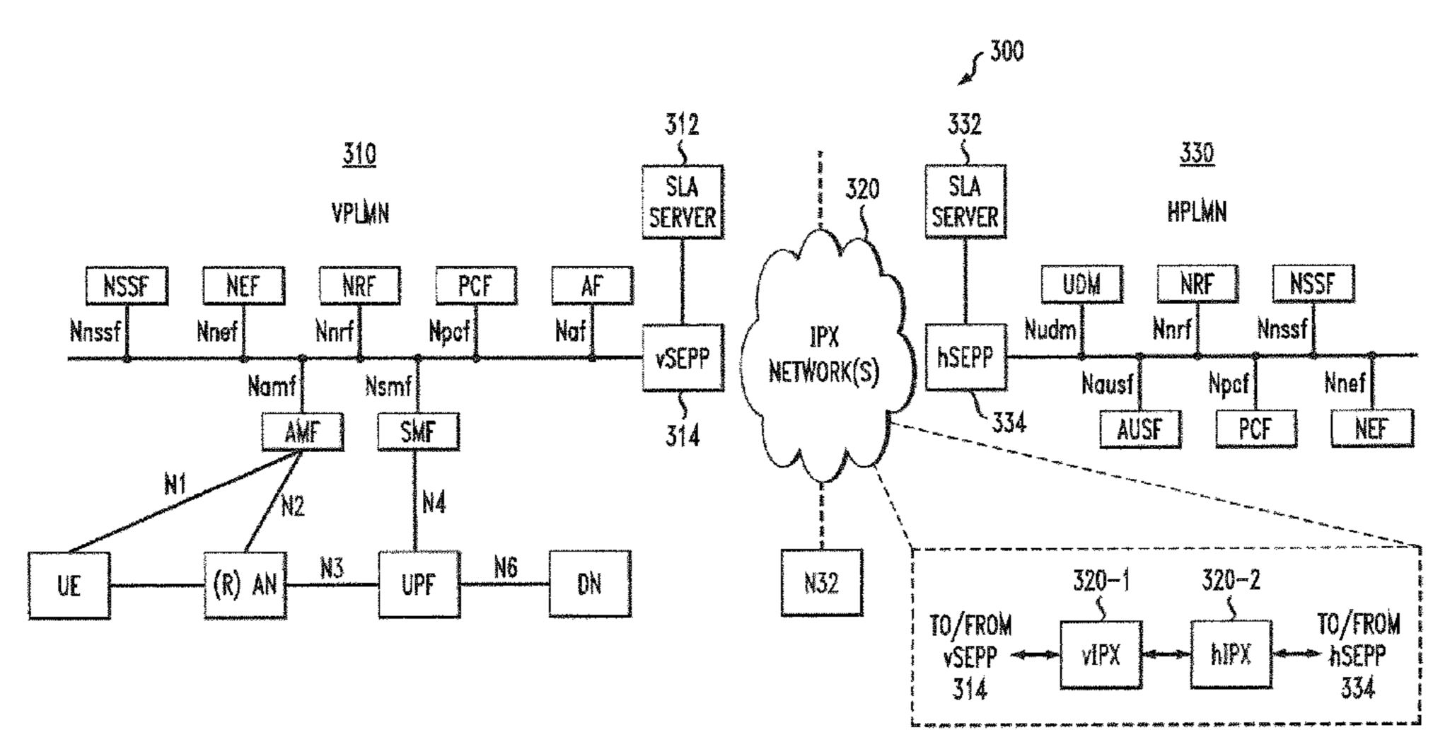
communication network. An automated verification of information in the message is performed at the first communication network to determine compliance with the service level agreement. The message receiving step is performed by a security edge protection proxy function of the first communication network and the automated verification performing step is performed by a service level agreement management function of the first communication network.
