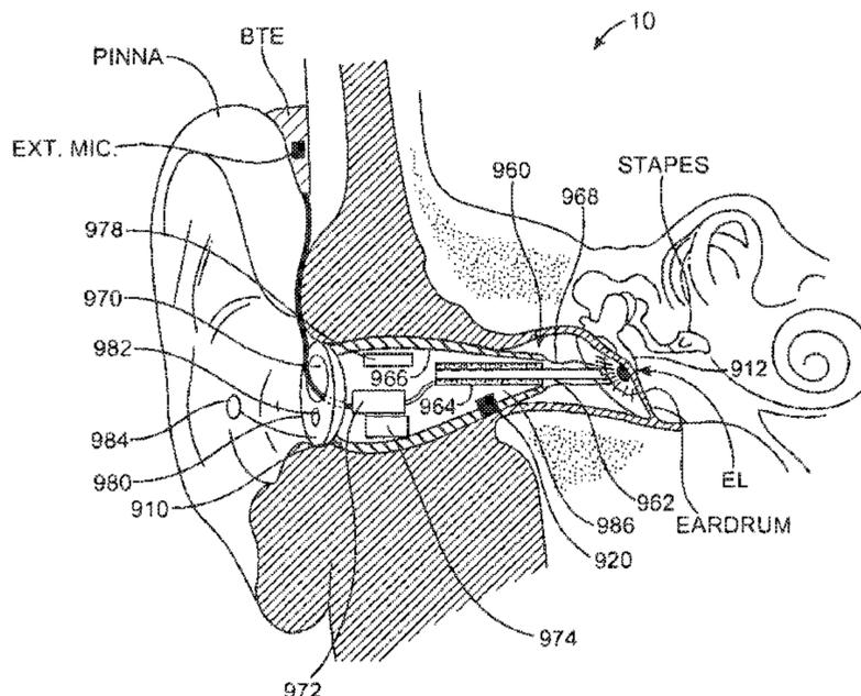
the user can receive and transmit audio signals. A bone conduction sensor can detect near-end speech of the user for transmission with the wireless circuitry in a noisy environment. Noise cancellation of background sounds near the user can be provided.
