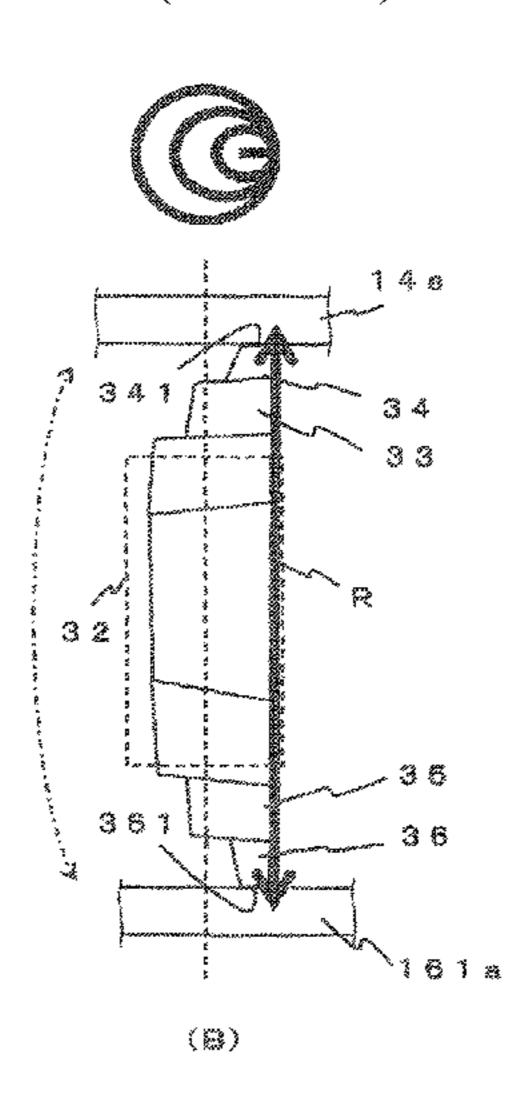
each of the first elastic portion and the second elastic portion by winding the main body, in which each or either of a tip end surface of the first contact portion that contacts the first contact target and a tip end surface of the second contact portion that contacts the second contact target is an inclined surface.
