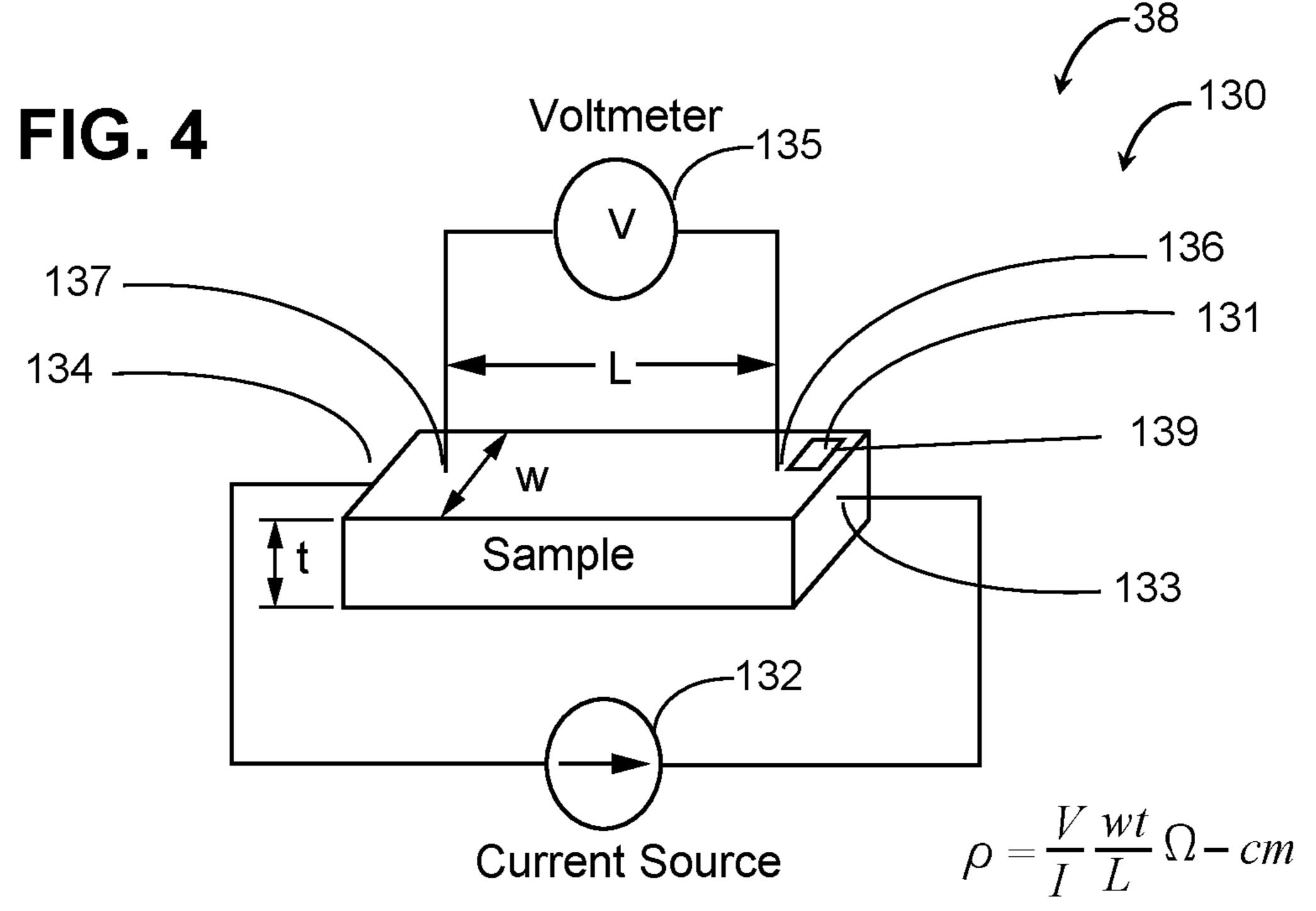
MEASURE THE RESISTIVITY OF THE BOILER WATERWALL FOR A SELECTED LOCATION UNDER KNOWN TEMPERATURE CONDITIONS.
